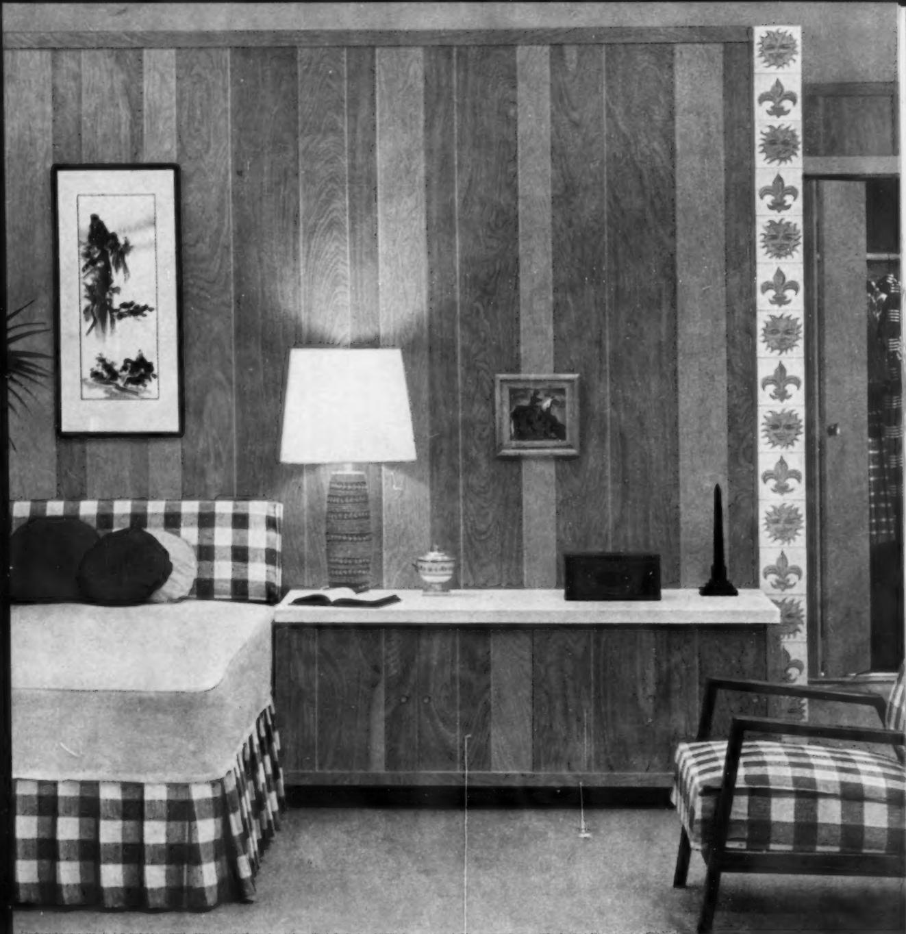
Wall is of 4' x 8' Birch V-Plank\* panels, with matching Weldwood hardwood moldings. Weldwood Bi-Fold closet doors (right) are birch-faced, have cores of non-warping Novoply.®
