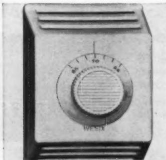
**COMBINED THERMOSTAT** and two-pole switch from Wesix. Model DLV gives sensitive direct control of electrical heating cable, of non-automatic heaters, duct heaters, other electrical heating units. Rated at 25 amps, 240 volts. Wesix Electric Heater Co., Dept. AB, 390 1st St., San Francisco 5, Cal. (No. 5016, p. 132.)
