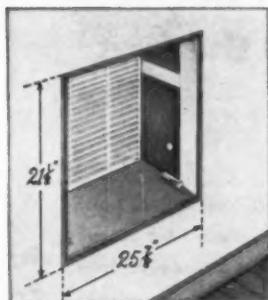
Case is installed during construction—mounts in any kind of wall. Panel protects opening until building is completed.
