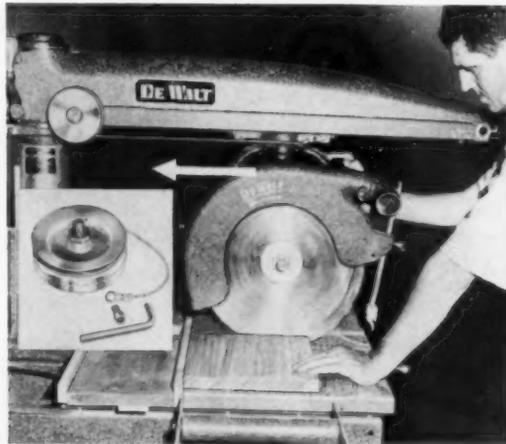
**SAFETY RETURN** device, De Walt Spir'Ator automatically returns carriage and cutting member of radial arm wood-working machines to rear idle position as soon as operator relaxes his forward pull on the motor carriage. The device, which is spring actuated, is made for De Walt by Hunter Spring Co., Lansdale, Pa. **Circle No. 10008.**
