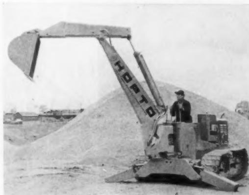
**HYDRAULICALLY ACTUATED OUTRIGGERS** are now built-in to this Hopto digger, Model 190 SPC-55. Operator can control each stabilizer individually for leveling machine on uneven terrain. Model has enclosed type boom and five-inch I.D. cylinders on hoist, crowd and bucket-actuating equipment. Digging depth of 11½ ft. and 190° swing; powered by Continental F226 engine. Badger Machine Co., Attn. Urban Shugart, Dept. AB, 1124 W. Fifth St., Winona, Minn. (Circle No. 10031 on page 154).
