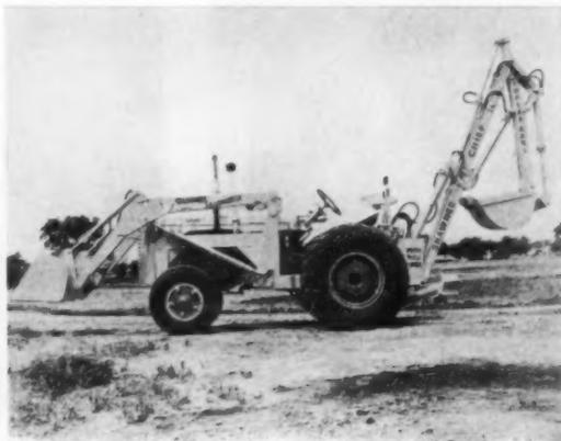
**BACKHOE DIGS A DEEP 14 FEET** according to its makers. Shawnee Mfg. Co. Model No. D90, the "Chief", actually reaches 15 ft. below the ground, has exceptional push-pull-power by synchronizing action of push cylinder at one end of the bucket boom with another pull cylinder midway between axis and bucket. Boom works in three 120° quadrants. Backhoe price: \$3,100 to 3,300. Shawnee Manufacturing Co., Attn. E. W. Avery, Dept. AB, Topeka, Kans. (Circle No. 10026 on card, page 154).
