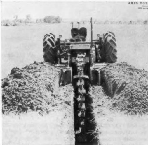
**TRENCH-HOG** is Arps low cost tractor attachment to handle big yardage jobs. It is available in three boom lengths, with digging depths of 3½ to 7'; cutters available 6 to 20" wide. **Circle No. 10002** on reply card, p. 134.
