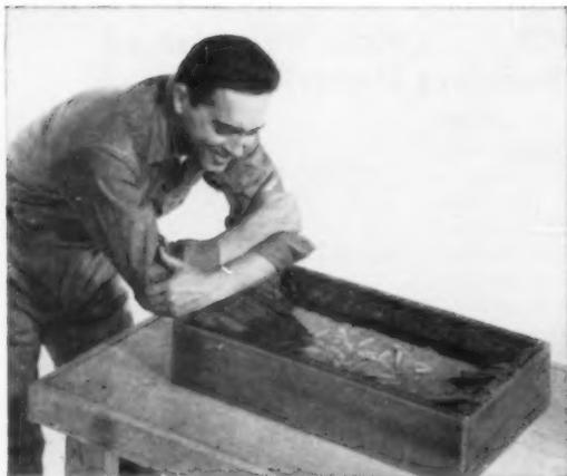
You can easily make this demonstration unit yourself! Just build a 24" x 12" frame out of 1" x 6" lumber. Staple 16" standard Balsam-Wool to the top, as shown. Fill with water—and for interest, add fish.
