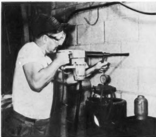
**POWER HAMMER**, under 13 lb., drills holes up to 1 1/8" diameter in toughest materials, Spring floated piston, neoprene mounted nozzle, induction hardened helical gears are featured in the Remington Rand H54U. It delivers up to 2300 blows per minute. The crank assembly is counter-balanced. Switch is sealed against dirt. **Circle No. 10007.**
