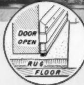
**DOWN** snugly against floor to seal out drafts when door closes.
