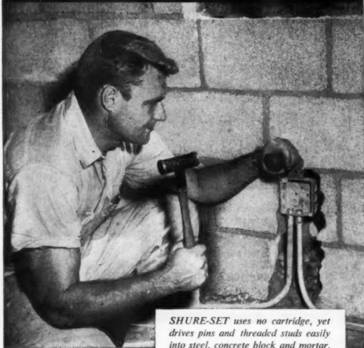
*SHURE-SET uses no cartridge, yet drives pins and threaded studs easily into steel, concrete block and mortar.*
