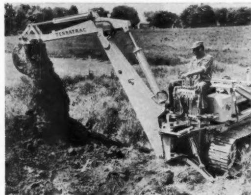
**180 DEGREE BOOM SWING** is one of the features of the new TerraTrac backhoe. Designed for heavy-duty use with TerraTrac crawler tractors, the 180° swing is done with hydraulic foot pedal control, enabling operator to maneuver bucket and dipper stick while swinging. Unit digs 12½ ft. deep, has 18 ft. reach and 13 ft. dump height. Easily detached when using front-mounted loader or dozer. From American Tractor Corp., Dept. AB, Churubusco (Ft. Wayne) Ind. (Circle No. 10030 on page 154).
