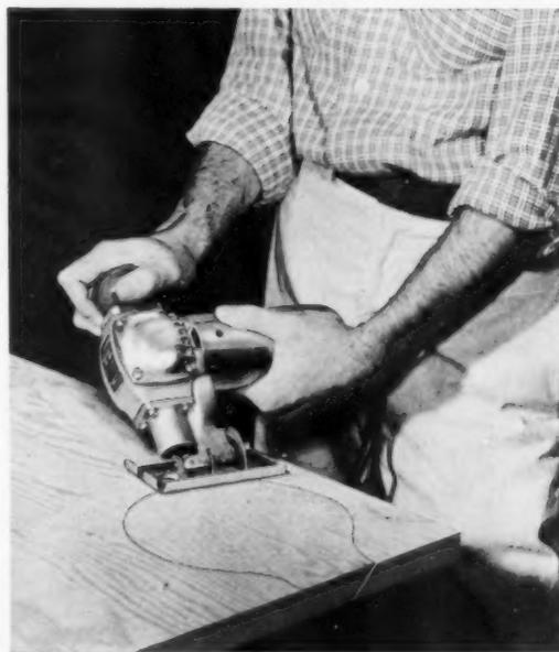
**BEVEL CUTS** on either side up to  $45^\circ$  is feature of Black & Decker jig saw No. 11. It has full one inch stroke; 2" depth at  $90^\circ$ ,  $1\frac{3}{4}$ " at  $45^\circ$ . Shoe adjusts to any angle. The weight of the Heavy Duty jig saw is 6 lb. A metal-cutting blade and three high speed wood cutting blades are included. **Circle No. 10012 on reply card, p. 134.**
