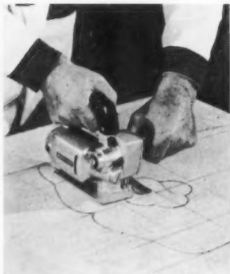
**BAYONET SAW** featuring orbital motion is recommended for economical and fast cutting of Formica, plastics, ferrous and non-ferrous metals, woods. Model 148's blade teeth contact material only on the cutting stroke. Lists at \$99.50. Porter-Cable, Attn. M. Nodar, Dept. AB, 1714 N. Salina St., Syracuse 8, N.Y. (No. 10022, page 154).
