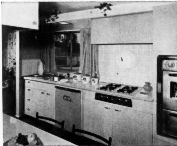
**KITCHEN** is corridor type. Cabinets are natural wood. Built-in oven and cooking top by Tappan, dishwasher by GE, disposer by Waste King; counter top by Never-Mar. Note soffit above sink, which holds indirect lighting.
