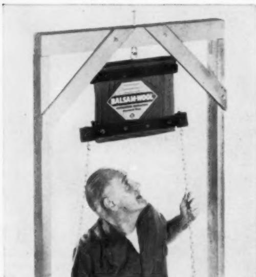
Here's a lively demonstration that drives home the ruggedness of Balsam-Wool insulation. Build a simple frame of 2" x 4" lumber; suspend a short length of 16" Standard Balsam-Wool from the top as shown. Add a "swing"...and you're ready to demonstrate just how tough Balsam-Wool is!
