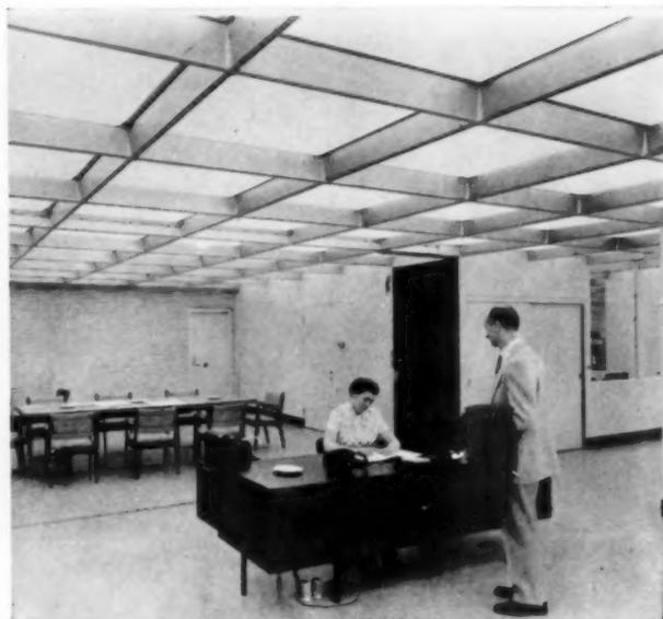
**FOUR-FOOT MODULE** of suspended ceiling is used throughout entire building. Light level is 100 foot-candles at wall. Ceiling is of acoustical baffles and plastic diffusers. Partitions are removable.
