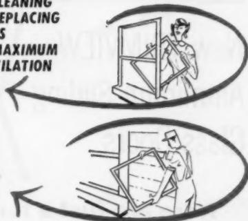
Window sash equipped with SNAP-TITE can be taken out or put in at any place. Balances engage automatically. SNAP-TITE can be used with standard frames and sash with only minor changes. The snap-in feature and complete factory assembled parts are designed for fast set up time.
