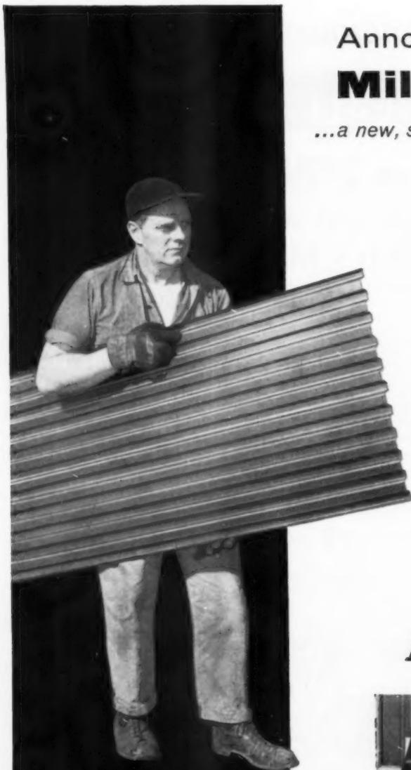
Milcor Ribform is a new, permanent, high-strength steel form for concrete floor-and-roof-slabs poured over steel joints or beams. It is quickly laid in sheets and welded to the steel supports where it becomes a rigid, non-porous base for the concrete.
