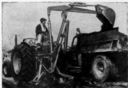
**F.M.D. Tractor and Digger** cuts costs of laterals, footings, service lines. Fast, positive hydraulic control. Fordson Major Diesel equipped with both rear-mounted backhoe and front-mounted loader makes an efficient, low-cost unit for excavating, loading, backfilling.
