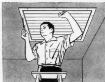
**Step 3.** Screw-fasten automatic ceiling shutter. Metal trim covers edges of opening. No finishing.
