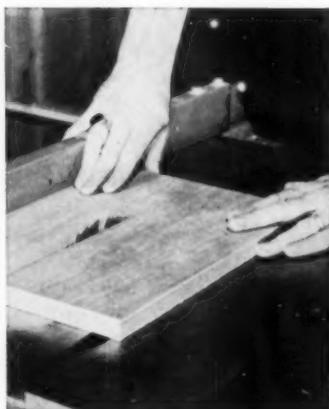
**2 POWER SAWING.** Face good grade of hp panel up when using bench saw. When both sides are good grade, as in cabinet doors, place a piece of scrap beneath plywood to prevent fuzzing the side that faces down.
