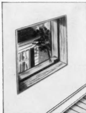
**Build sleeve and frame into wall during construction.** Opening is about 27" wide, 23" high. More through-the-wall units can be added later.
