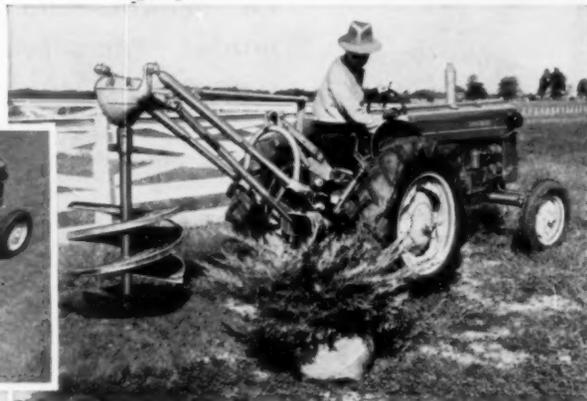
Above—The Utility Tractor and Power Hole Digger—today's easy method for digging holes for posts, guard rails, tree settings, and construction work. Digs as deep as 40 inches; several auger sizes.
