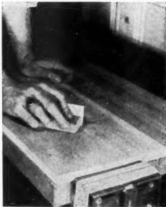
**4** **SANDING.** Run *with* the grain, not across it. Start with medium sandpaper and work down to fine grades to get finishing surface. Be sure to remove dust. Since hp is pre-sanded at mill, little sanding is needed.
