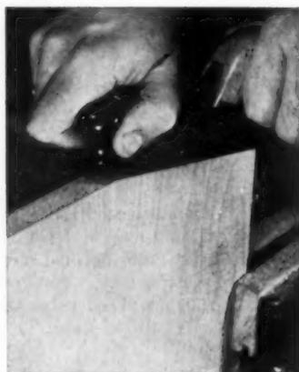
**3 PLANING.** Hold the plane in angled position as it runs along the plywood edge. Never run plane off the end of the edge. Instead, turn plane around and begin at that end to level up the cut.
