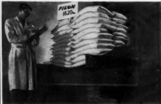
**FILON HAS MUCH HIGHER LOAD CAPACITY THAN REQUIRED BY STANDARDS OF THE INDUSTRY.** Shown above is a 26" wide FILON type 250 panel over a 4" span supporting a static load of 1820 lbs.—equivalent to 210 lbs. per sq. ft. Compare this with the 100 lbs. per sq. ft. required by industry standards.
