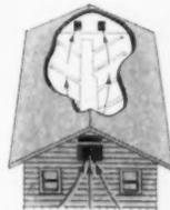
**PULL-THROUGH DESIGN**—Air is pulled through condenser which traps rain—keeps unit and electrical components dry. Operation is quieter, efficient. Exhaust air can be discharged into attic for forced air circulation at no extra cost.
