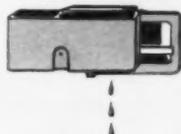
Meanwhile, water collects in both tanks. At the end of the first wash, it automatically drains out through a small hole in one of them.
