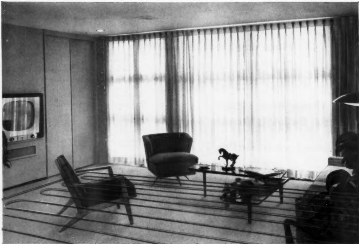
**SUPERIMPOSED** on the photograph of the living room, in one of the homes of the Crabapple Court tract, is a section of the radiant panel heating system. With radiant panel heating picture windows can be brought right to the floor line, allowing a free reign in interior decor and furniture arrangement. And with radiant heat there are no drafts, no hot and cold zones.
