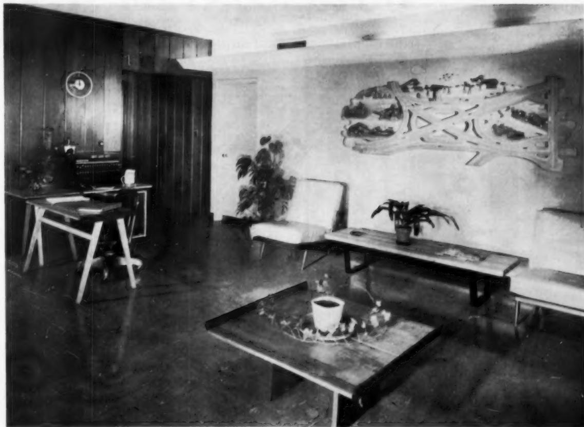
**INTERIOR PARTITIONS** are wood framed, with walls finished in combinations of plaster and vertical wood veneer planking
