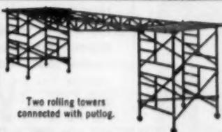
Two rolling towers connected with putlog.
