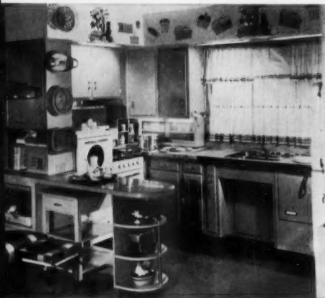
**THE STORE-IN-PLACE PRINCIPLE** can make better sense out of a breakfast bar. Leaving the center portion under the counter open permits storage of a small serving table, as well as knee room when counter is used for other purposes.
