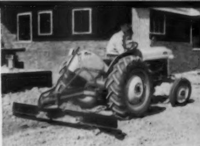
**BETTER BLADING AND BACKFILLING**—Equipped with a rear blade, the Ford Tractor is well suited for grading, ditching, backfilling and aggregate mixing. Fast, easy hydraulic operation.
