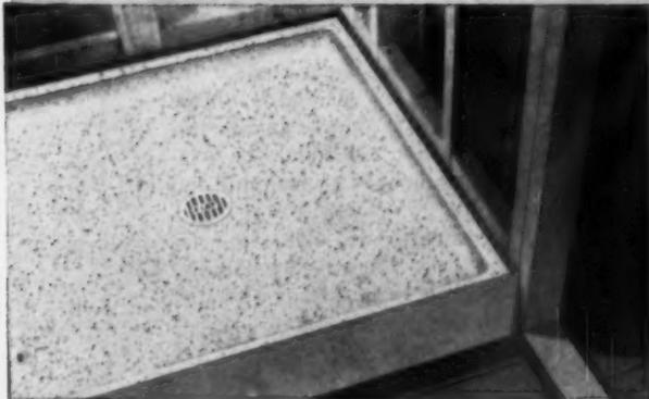
**2** The shower floor slides into place. It is a self-contained, monolithic unit with both metal tiling-in flange and drain cast integral. Plumber makes calked drain connection quickly and easily while installing floor. No call backs—no other trades required—ideal with any wall material.
