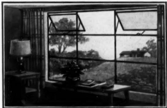
Hope's New Roto Ranch Windows have wide (1 $\frac{1}{2}$ " muntins in proper proportion to panes. They provide great rigidity and harmonize with residential construction. Awning type ventilators open and close easily, quickly. Die-cast underscreen roto operator has extension arm of stainless steel fitted with a bronze shoe.
