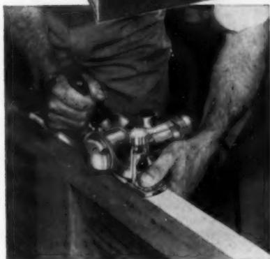
Power Plane quickly trims doors, windows and storm sash to fit; Router makes hinge mortising better and easier; Butt Templet guides Router
