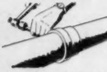
Joints of cast iron pipe are packed with oakum and caulked with molten lead. This combination provides a joint that absolutely prevents root penetration.
