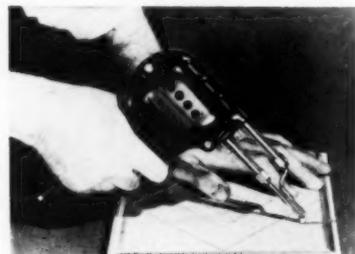
flat metal or glass surface. Manufacturer states that tool will also cut asphalt and rubber tile, linoleum and like materials.
