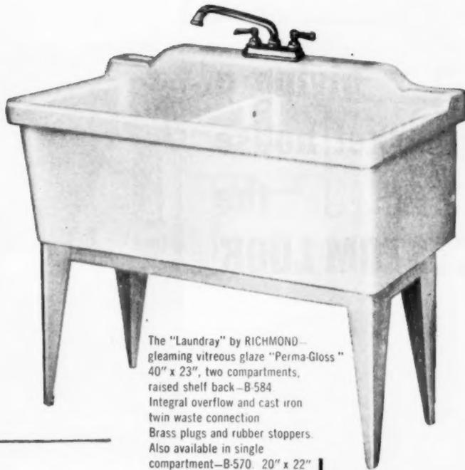
The "Laundray" by RICHMOND—gleaming vitreous glaze "Perma-Gloss" 40" x 23", two compartments, raised shelf back—B-584. Integral overflow and cast iron twin waste connection. Brass plugs and rubber stoppers. Also available in single compartment—B-570. 20" x 22"
