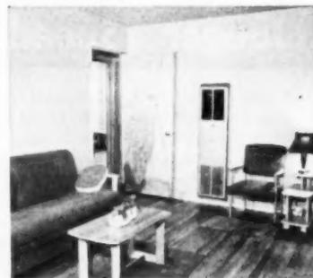
Living room is 12x18 feet. Oak flooring is an extra; standard model has asphalt tile laid over slab floor. Note the gas-fired wall furnace
