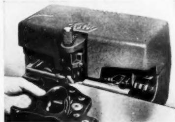
precision results from the "twin-hammer" action, both hammers being powered by a single spring. Only three adjustments are needed for automatic operation: insert the saw, select the points per inch (from four to 16), and adjust the depth of set. No special skill is needed for accurate operation.
