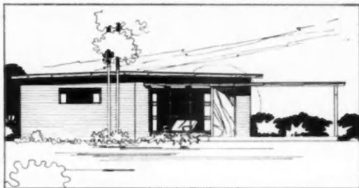
Combination rafter-joists give pitch to the roof and a level ceiling in this elevation. This is made possible by ripping 18-foot 2x14's diagonally to get two 18-foot pieces 4 inches wide at one end and 10 inches at the other. The 10-inch widths are placed at the ridge
