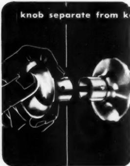
Forcing knob with wrench or tool will not open locked door. Knob is absolutely separate from lock mechanism. Knob slides on cam... then is firmly held in position by spring retaining pin.
