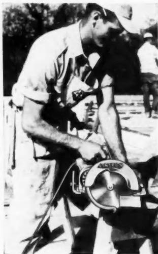
The new Dual V-Belt Drive eliminates gears—provides shock-absorbing, velvet smooth operation for faster, cleaner cutting. Cuts and rips wood; cuts and scores brick, tile and other materials with 6000 RPM full load blade speed. Its high speed feeds the blade in—no need to push or ram. The powerful motor—full ball-bearing . . . exceptionally cool—develops up to 1- $\frac{1}{2}$  H.P. It weighs 19 lbs., just the right weight for its 8- $\frac{1}{2}$ " blade and 2- $\frac{11}{16}$ " cut.
