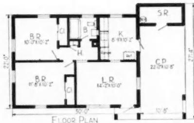
**TWO-BEDROOM FLOOR PLAN** features compact room arrangements with little lost space. Both bedrooms have steel, sliding-door wardrobes. Storage and utility room is located at the rear of the carport.
