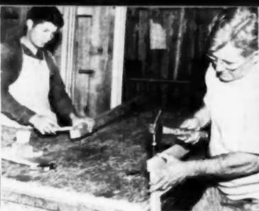
**TWO MEN** assemble sliding doors for wardrobes. One spreads glue on stiles, starts nails. Second man puts cabinet together, sets nails. Avoids making one man handle glue pot, nails and two stiles
