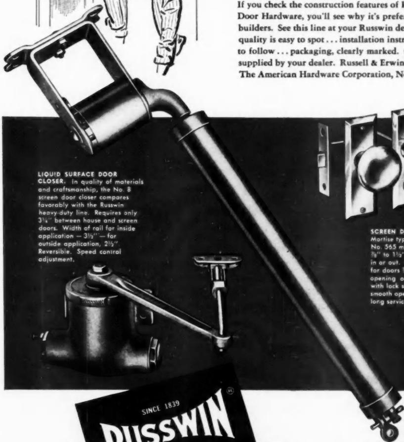
**LIQUID SURFACE DOOR CLOSER.** In quality of materials and craftsmanship, the No. 8 screen door closer compares favorably with the Russwin heavy-duty line. Requires only 3 1/4" between house and screen doors. Width of rail for inside application — 3 1/2" — for outside application, 2 1/2". Reversible. Speed control adjustment.
