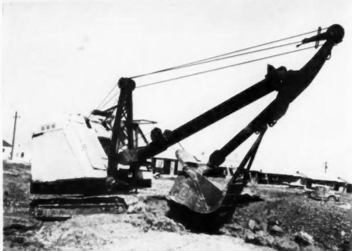
VALUABLE ON ROUGH TERRAIN, this track-operated model 70 Buckeye back-hoe digs service lines
