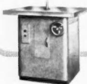
Whitney 510 SHAPER — Belted, motor drive. Table, 36" x 31". Vertical adjustment of spindle, 3 1/2". Detachable spindle top.
