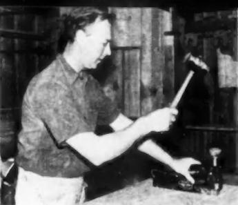
**STAPLING** plywood to wardrobe frames. Three rows of staples six inches apart go in faster than 60 a minute by hitting Spotnailer stapler with rubber mallet. No countersinking necessary
