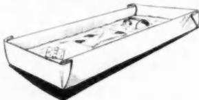
A simple container for cleaning a miscellaneous assortment of articles on the job may be made from a single piece of building paper. This should be placed in a hole in the ground of the same size. Building paper is folded at corners in the manner shown in the drawing.
