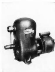
**AB12466 — TANKLESS WATER SYSTEM** — Goulds Pumps Inc., Dept. AB, Seneca Falls, N. Y. The Close-Cuplid Balanced Flow jet is a self-contained, shallow-well water system that operates without storage tank. Pump capacity is 520 GPH at 10 foot suction lift. Measures 20 by 11 1/2 by 15 inches over-all. Rotating impeller only moving part.
