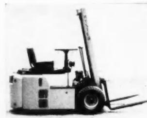
**AB12289—LIFT TRUCK**—Hyster Company, Dept. AB, 2902 N.E. Clackamas St., Portland 8, Ore. Company reports engineering changes in Hyster's Model '20' lift truck are a new upright assembly and new load arm pins which will permit the use of optional additional counterweight on the standard 2000-pound capacity model, (shown above) thus increasing or decreasing load-center or load capacity as the need requires. Photo shows extra demountable counterweight "pads" on back.
