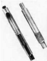
**AB12435 — STUB NAIL DRIVER** — Steelcrete Magnetic Punch, Howard Van Orden, 141 Godden Ave., Paterson, N.J. A new device for driving stub nails into concrete, stone or steel has been developed by a union fitter, Van Orden, and endorsed by the Metal Lath Mfg. Association. The device enables metal lathers to safely use stub nails.
