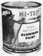
**AB12210 — ALUMINUM PAINT** — Illinois Bronze Powder Co., Dept. AB, 2023 S. Clark St., Chicago 6, Ill. Hi-Temp paint withstands heat as high as 1200 degrees F. No special surface preparation is required. One coat covers by brush or spray, and the paint dries in 1 to 2 hours. Effective on furnaces, boilers, ovens, steam pipes, etc.
