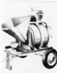
**AB12341 — AUTO-LOADER** — Jaeger Machine Co., Dept. AB, Columbus, Ohio. The hopper can be loaded while batch is mixing, then it automatically shakes load into the drum. This makes it possible to produce 12 to 15 more yards of concrete daily. Gasoline powered. Drum is mounted on steel tracks.
