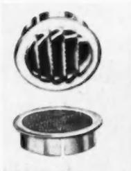
**AB12190—MIDGET LOUVERS**—Midget Louver Co., Dept. AB, Norwalk, Conn. A simple device to enable fresh air to circulate through walls. Used at eaves, gables, dormers, porch floors, storm sash. Installed simply by drilling hole and inserting. Helps correct paint blistering. Made of aluminum in sizes of 1, 2, 2 1/2, 3 and 4 inches.
