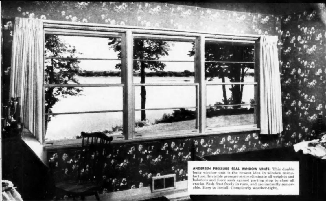
**ANDERSEN PRESSURE SEAL WINDOW UNITS:** This double hung window unit is the newest idea in window manufacture. Invisible pressure strips eliminate all weights and balances and force sash against parting stop to close all cracks. Sash float freely in runs, and are instantly removable. Easy to install. Completely weather-tight.
