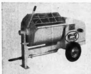
**AB12114-PLASTER MIXER**—Muller Machinery Co., Dept. AB, Metuchen, N. J. The 3 cubic foot plaster and mortar mixer recently introduced by Muller, is now equipped with a neoprene seal to eliminate wear on the paddle shaft. The small Muller mixer is built along the same heavy-duty lines as the larger machines, according to the company. Convenient loading height is 32 inches and a width narrow enough to go through a 30-inch door. Also available in 6 and 9 cubic foot sizes. Gas or electric powered.
