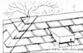
If the roof has large overhangs ventilation can be secured by cutting holes into the underside of the soffit. These will need screening to keep insects from entering the house. Small, metal louvers of 3-inch diameter are manufactured for this purpose and are easy to install. If the roof does not have any overhang then a roof type ventilator can be installed.
