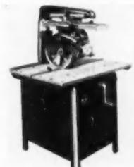
**AB12105—RADIAL SAW** —Delta Power Tool Division, Rockwell Mfg. Co., Dept. AB, Milwaukee 1, Wis. Three HP Delta Radial Saw cuts 3 1/4 inches thick and has a 19 inch saw travel. Exclusive 360 degree radial action design allows performance of any angle cut. Controls are located in front for easy reach. Booth 13, Stevens.
