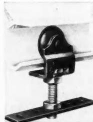
**AB12160—SLIDING DOOR HANGERS** — Richards-Wilcox Mfg. Co., Dept. AB, Aurora, Ill. A line known as "Silver Strak" hangers and designed for use on doors ¾-inch or more in thickness and weighing 100 to 200 pounds. They attach either to the top or face of the door and have Oilite self-lubricating bearings.
