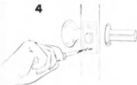
4 Fasten face plate with 2 wood screws.
