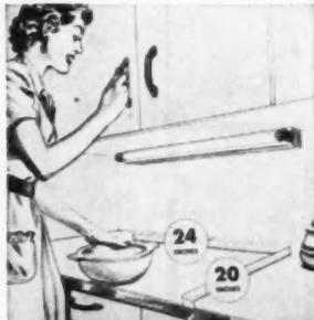
ONE of the most popular features of Light-Conditioned kitchens is the light over the sink. This can be accomplished by installing two 25-watt fluorescent units, a 75-watt floodlight bulb or a 150-watt standard lamp bulb in a 12-inch enclosing globe
