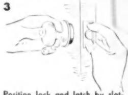
3 Position lock and latch by slot-engagement.
