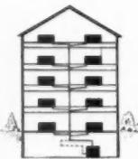
**Damper Modulated Heat Delivery for Comfort and Economy** — Personalized room temperature control by manual adjustment of convector dampers eliminates expense of valves . . . discourages wasteful over-heating. When valves are used on 1-pipe steam radiators, they must be of the "on-and-off" type which do not permit modulation of heat delivery. *Only convectors offer this important refinement in 1-pipe steam heating.*
