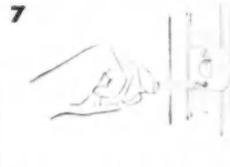
7 Fasten strike plate with 2 wood screws.
