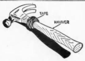
**TAPE** wrapped around the handle of hammer near the head makes it easy to pick up.—Geo. Wilson, New Haven, Conn.
