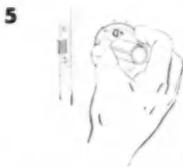
5 Put on clamp plate by turning to engage keyway. Tighten screws.
