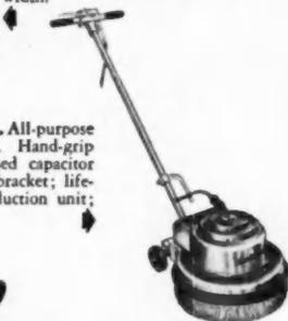
**HOLT WHIRLWIND SPINNER.** Heavy duty, super-powered. Five tools in one — sands, wire brushes, grinds, planes and bevels.
