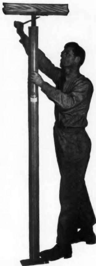
**1. CAP AND BASE PLATES** are flat (not embossed), 1/4" thick, have a 4" x 8" surface, carry safe, usable loads of 12,500 pounds; maximum to 22,000 pounds (more than average residential use). Slotted holes in cap plate for bolting to steel beams; separate nail holes for wood beams.
