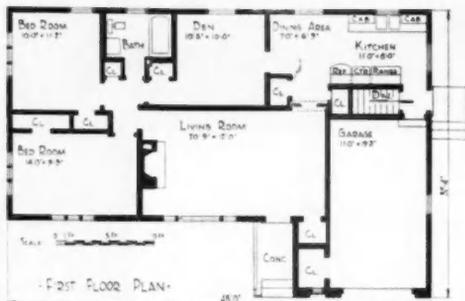
PLAN with attached garage is designed for 66 foot lot
