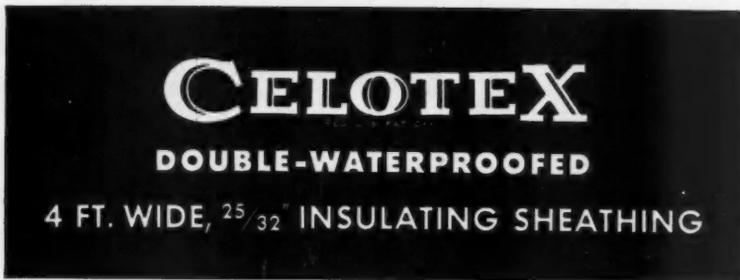
You can eliminate the expense of corner bracing... yet build better, stronger walls... with 4 ft. wide,  $\frac{25}{32}$ " thick Celotex Insulating Sheathing! Without corner bracing it greatly exceeds rigid F. H. A. requirements, which call for bracing strength at least equal to horizontal wood sheathing with corner bracing. Official test results at right prove it!
