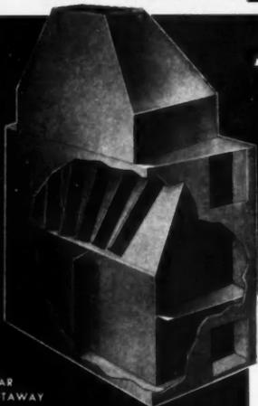
Note wide *Radiant Blades* within the heating chamber. Solidly welded to firebox, these metal fins boost heat-radiating surfaces and guide air over unit's hottest area.
