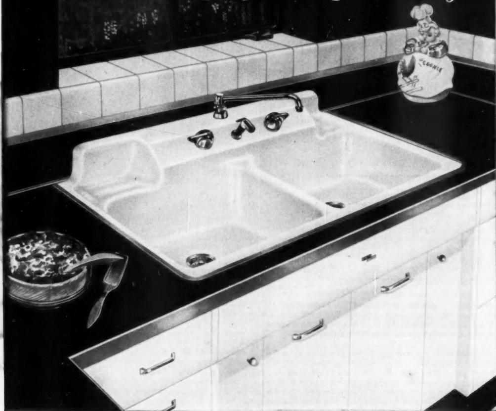
**ALL-AMERICAN COUNTER-TOP SINK.** One-piece construction of porcelain enameled cast iron—in white and eight Crane colors. Two 8-inch deep basins, 17" x 15½". Four-inch high back. Chromium-plated trim includes *Dial-ese* controls, swinging mixing spout, retractable hose spray. Overall size: 38" x 22". Consult your Crane Branch or Crane Wholesaler.
