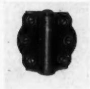
**Screen Door Hinge**—Stanley Works, New Britain, Conn. New adjustable tension screen door hinge has spring adjustable to regulate speed of closing. Spring is in barrel of hinge. Made of wrought steel for half- or full-surface applications.
