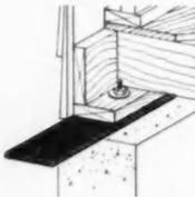
**Sill Sealer**—The Celotex Corp., 120 S. LaSalle St., Chicago 3, Ill. Flexcell, 8-inch wide, 1/2-inch thick, forms excellent seal between foundation and sill plate to minimize heat loss and wind infiltration. Not affected by termites or fungus.
