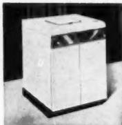
**Automatic Washer**—Blackstone Corp., Jamestown, N. Y. Model 150 washer has precision-built driving mechanism, with hardened steel gears, rubber-mounted on welded steel chassis. Stainless steel tub is 20 inches in diameter.
