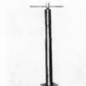
**Adjustable Basement Post**—The Sawhill Mfg. Co., Sharon, Pa. "Red-I-Post" has patented Ring-Lock which bears upon full circumference of two telescoping columns, distributing load uniformly, preventing spreading or mushrooming.
