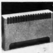
**Convecter**—John J. Nesbitt, Inc., State Rd. and Rhawn St., Philadelphia 36, Pa. Radiates heat moderately. Principal mode of heating is convection of air from floor level, through fin-and-tube heating element and out grille.
