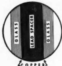
**A:** A continuous strip of copper is bonded to the inner surface along the edge of each pane . . . then the lead spacer is heat-bonded to the copper alloy. Glass, copper band and lead spacer are joined into one strong, solid unit.
