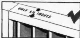
"WALL-FIT" THICKNESS—FOLDOOR occupies the least amount of "stack" space of any extensible door. When pushed back onto itself, FOLDOOR'S maximum thickness is only 5½ inches. This means FOLDOOR fits inside the measurements of most walls—does not stick out into the room.
