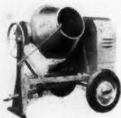
**Tilting Mixer**—Jaeger Machine Co., Columbus 16, Ohio. "Speedy" 3 $\frac{1}{2}$ -S side-discharge concrete mixer has patented V-bottom. Drum turns on two Timken roller bearings, is chain driven by 3 $\frac{1}{4}$  H.P. Wisconsin gasoline engine. Balanced for towing.
