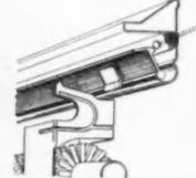
**Baseboard Heating** — Warren Webster & Co., Camden 5, N. J. New baseboard units have optional addition of manually operated damper to reduce heat flow in some rooms. Magnesium alloy damper fits into groove in Webster metal molding.
