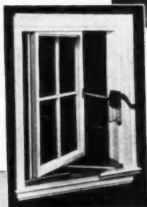
● **A COMPLETE UNIT**—with all parts pre-fitted—consisting of frame, sash, all operating hardware, insulating glass, screen and Mitertite trim. The illustration shows small unit with part of trim cut away to show how operating mechanism holds sash firmly in any position without rattling, swinging or vibrating.
