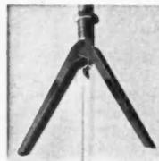
**Fixture Hanger**—Paine outlet box and fixture hanger consists of two wings, each mounted on a ¾-inch nipple which is 2¼ inches long. A key locks wings when they are open. Made by Paine Co., 2947 Carroll Ave., Chicago 12, Ill.
