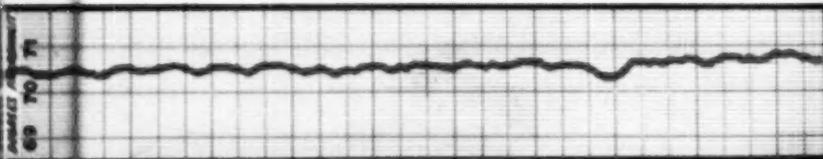
Temperature reading from the new Honeywell TM Comfort Thermostat, both recordings made under almost identical conditions.
