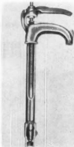
Ratchet type handle provides seven speeds in a half turn on new JK non-freezing ground hydrant designed for use with stock tanks and other places on farm where water pressure is provided. Shut-off valve below frost line is controlled by valve rod in inner pipe. Special outlet drains water left in pipe after shut-off. Space between faucet and ground measures 36 inches. James Knights Company, Sandwich, Ill.
