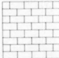
**ESPECIALLY good for large rooms, ashlar patterns may be obtained by the staggering of joints**
