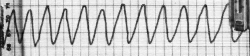
Temperature reading from conventional heater type thermostat.
