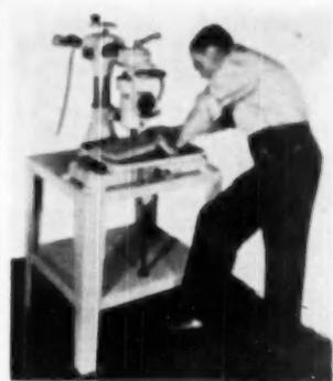
ROUTING with the versatile Comet Cub may be done free hand, against the shaper fence or with a template. Foot-operated, the router table can be accurately set for depth of cut with special micrometer depth-adjuster
