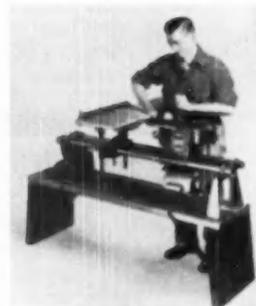
lath, 17-inch disc sander, or horizontal drill press. The horizontal drill press, shown here, is a new power tool for jobs such as doweling, drilling in the ends of long workpieces, and other jobs that are difficult or impossible on a vertical drill press. Accessories can be added to convert into a jointer, shaper, drum sander, moulder, jig saw, and other power tools. Magna Engineering Corp., Dept. AB, 417 Montgomery St., San Francisco, Calif.
