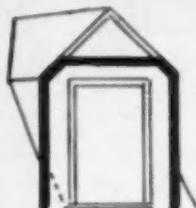
**ALL** dormers should be insulated with special care. The entire surface of the exposed walls as well as the ceiling sections must be encased with insulating material. All narrow spaces around windows should be carefully packed to assure maximum efficiency
