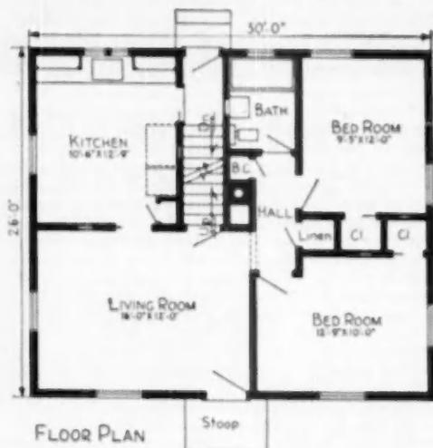
BASIC plan for all houses. Stair area is converted to closet in house without attic
