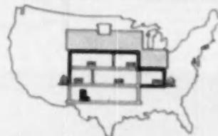
**IN DEVELOPING** a yardstick to measure the comfort rating of a home, it is generally recognized that 70 degrees is the accepted indoor temperature in winter. Because the outdoor temperatures fall to 0 or below in most areas of the United States, insulation is required to keep the inside surfaces of exterior walls within a few degrees of the room temperature. If these surfaces are more than 6 or 12 degrees colder than the air, rating is poor
