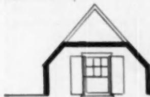
**INSULATION** should form an envelope to separate the heated rooms of a house from the unheated porches, garage, attic and crawl space. If the attic is not used, insulation should be placed in the attic floor. If a room is built in an attic or low upper-story area, insulation should be installed in the walls and ceiling by following the outline of the room. Flow of air from the eaves to gable or ridge louvers should not be blocked at the knee walls
