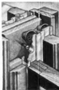
The exclusive spring cushion construction (cutaway view at left) not only makes the removable feature possible, it automatically adjusts to suit the weatherman. Gives in warm damp weather—expands in cold dry weather. Wood sash travel in metal sash guides for smooth operation.
