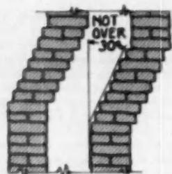
IF it is absolutely necessary to offset the flue, the angle of offset should never exceed 30 degrees. Less offset is even more desirable for greatest venting efficiency
