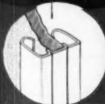
**SIDE TUBES\*** Made of rust-resistant steel, the 1" square tubes provide added reinforcement for rigidity of panels. **PANELS**... Smooth Masonite Tempered Presswood can be economically painted, stained or papered as desired for beautiful decorative effect.
