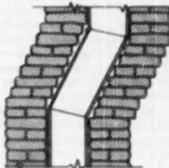
PROPERLY mitered joints where the flue lining sections join at both top and bottom of incline retain full flue area and reduce turbulence. All lining joints should be made perfectly smooth and tight
