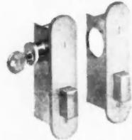
For narrowest extruded aluminum, structural steel and wood stiles Series 970 Deadlocks for standard cylinders have 1 3/8" backset, 1 3/8" depth. Fifteen other standard backsets to 1 3/4". Series 980 identical
