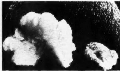
**PROCESSED** perlite aggregate, left is about six times the size of raw ore, right
