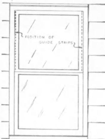
Above illustration shows top and bottom storm sections in position. No hardware is exposed or visible from the outside.
