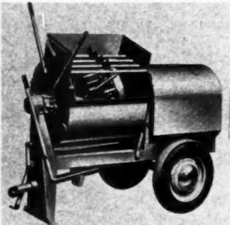
mixing drum and power plant separate, the unit is readily maneuvered about on the job. Handle-lever control of discharge at any point in arc of drum's tilt, with two discharge position—24 inches for wheelbarrows, and 17½ inches for mortar boxes. With axles telescoped and hub caps removed, mixer will pass through 33-inch doorways. Air-cooled, 6.4 H.P. gasolined engine. Jaeger Machine Co., Columbus 16, Ohio.
