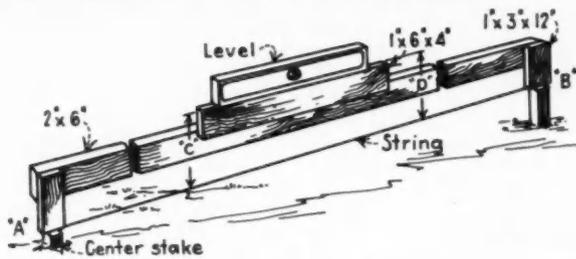
**W**HERE an instrument is not available for leveling a plot of ground, this home-made level can be used with excellent results.
