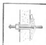
When hanging objects that must be moved periodically, use a nut and washer as shown above.
