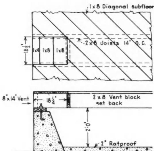
**I**N basementless houses with crawl spaces under first floor, an occasional ventilator is placed on the outside wall at the end of joist openings.
