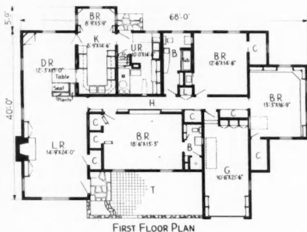
**FLOOR** plan shows successful utilization of space. Notice storage walls between master bedroom and hall, kitchen and dining area. Sliding doors were used wherever practical. Markey and Hoke planned 103 built-ins for this Bryan, Ohio, home
