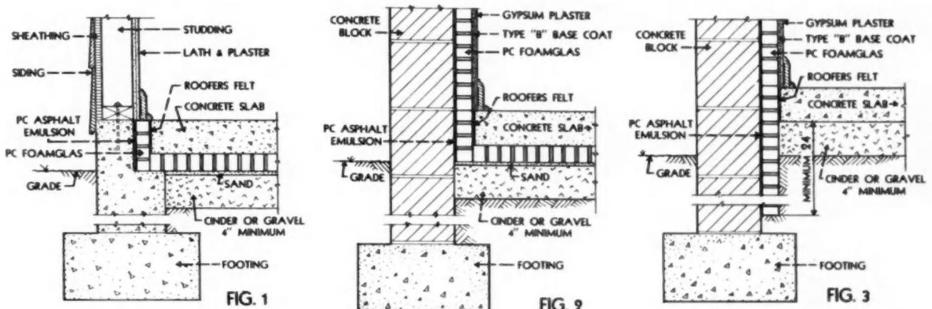
DRAWINGS showing alternate installation of glass insulating material as applied between wall and concrete slab around perimeter of structure. Each of these methods is sound in application, the builder's choice depending on adaptability to local conditions
