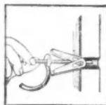
Just drill a hole. Unscrew wing. Put bolt through item to be fastened. Thread wing back on bolt. Push wing through hole.
