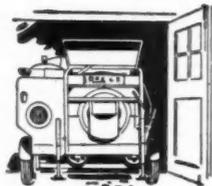
only 87 inches with skip up and 72 1/2 inches with skip down . . . permits working in restricted areas and allows for plenty of headroom for parking in garage or other buildings.
