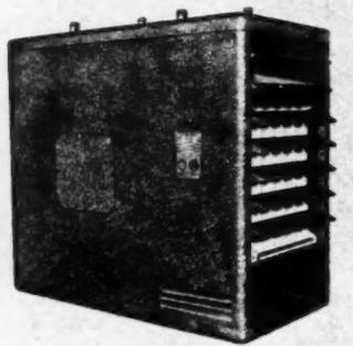
cage fan. In five sizes, with AGA output of 172,000; 136,000; 112,000; 84,000, and 68,000 B.T.U. per hour. Equipped with cast iron heat exchanger and combustion chamber to withstand corrosive effects of burning gases. Combustion chamber and heat exchanger are cast in one piece, and extended heating surface fins on heat exchanger are cast integral. Built-in draft hood absorbs all excessive chimney action. Automatic Gas Equipment Co., 301 Brush-ton Ave., Pittsburgh 21, Pa.
