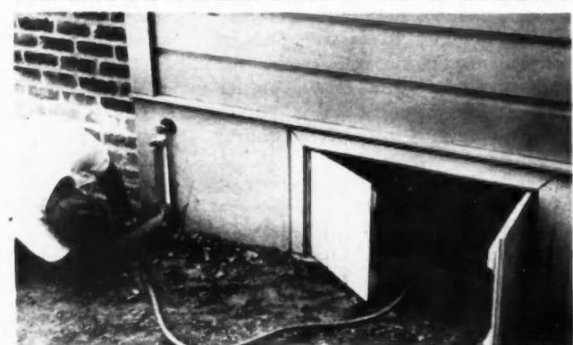
HOW much each part of foundation rises from original position is measured by this instrument. This knowledge will be used in experimenting with materials to use with clay soil that moves
