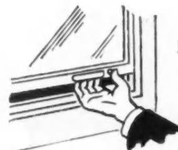
Slight pressure with thumb on side of handle releases lock so panel can be raised to any level. Release of pressure locks window . . . no weights, cords or spring balances.
