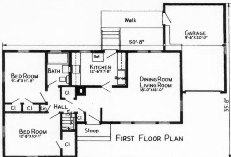
FLOOR plan of the I-E house with modifications developed as result of experience in building and selling the unit to customers in northern New York state area. A major alteration, not shown here, was in changing roof pitch from 5/12 to 8/12
