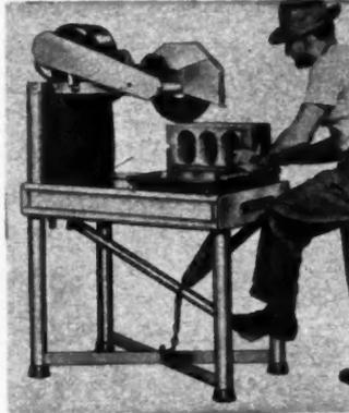
machine weighing 225 pounds. The 1½-H.P. motor drives both water pump and blade to make an efficient dry and wet cutting device. Available also in dry-cut models. Model knocks down to fit most automobile trunks. The Victor Engineering Corp., Bristol, Pa.
