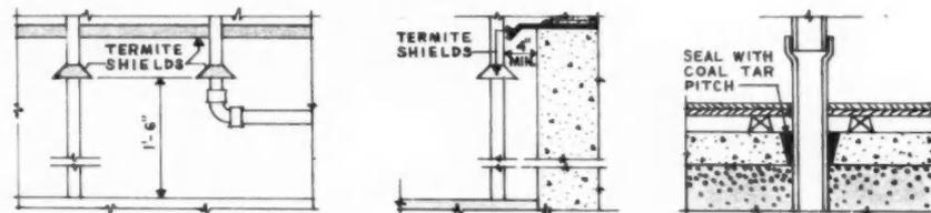
**PIPES ENTERING OR WITHIN 1'-6" OF GROUND OR THROUGH FLOOR SLAB**
