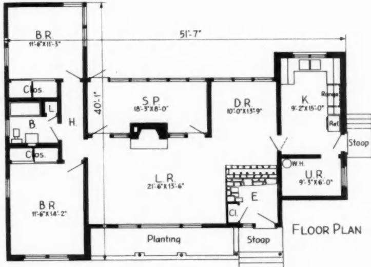
PLAN provides separation for services, plus exterior and interior planting
