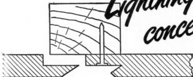
This J-M feature speeds alignment and offers the important advantage of concealed nailing. No exposed nailheads to mar the beauty of wall or ceiling. Beveled edges provide a neat "V" groove at the joints. Write for new brochure on J-M Decorative Insulating Board. Johns-Manville, Box 290, N. Y. 16, N.Y.
