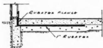
strength of 40 pounds per square inch. High resistance to moisture and vapor. No added water vapor barrier required. Rot, vermin and termite proof. Easily worked with ordinary woodworking equipment, either hand or power operated. Can be cut with a circular saw, band saw or hand saw. Great American Industries, Inc., Rubatex Div., Bedford, Va.
