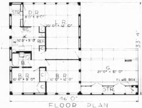
**PLAN** at left contains large central area with abbreviated partitions causing rooms to actually flow into one another. Carport at front doubles as porch. Storage units on one wall form barrier to house
