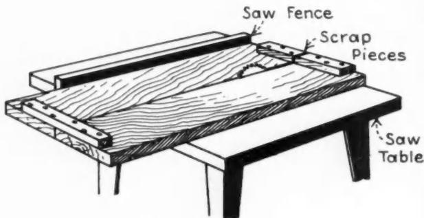
TAKE the two boards that are to be glued together and place them side by side and secure them temporarily top and bottom with scrap pieces. The scrap pieces are to be secured into the waste part of the boards to be glued.
