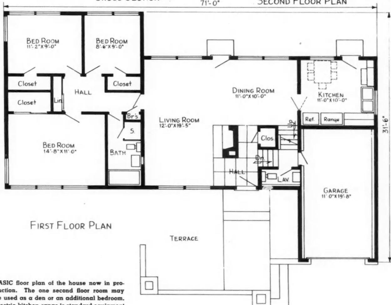
BASIC floor plan of the house now in production. The one second floor room may be used as a den or an additional bedroom. Electric kitchen range is standard equipment
