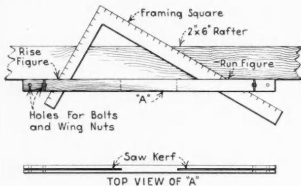
**A** HOMEMADE fence will prevent making mistakes when laying out a pattern for long rafters, when using the step method with framing square.
