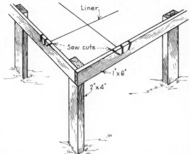
**H**ERE is another method of placing the liner on batter boards. In this way there is no danger of losing the liner as long as the batter boards are in position. To operate, place line through plumb saw cut and then loop through angle saw cuts to tighten line.—Submitted by Richard H. Barnes, Colwyn, Pa.
