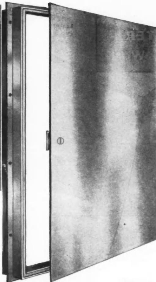
Ready to install • No special framing • Painted with rust-inhibiting prime coat • Concealed hinges • Flush, screw-type lock • 11 sizes — from 8 3/8" x 8 3/8" to 24 3/8" x 36 3/8" • For plastered or non-plastered walls • With or without expanded metal wings
