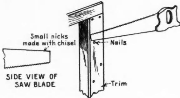
WHEN doing repair jobs it is often necessary to remove some portion of the work in as simple manner as possible; for example, the sill or sub-sill of a window frame or a section of trim. This can be quickly and easily done by using slightly altered tools for the purpose.
