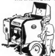
for fast operation at the end of the day as well as the start. Grouped controls swinging through short arcs cut operator fatigue. Skip clutch, brake, water valves and discharge controlled without moving from one spot.
