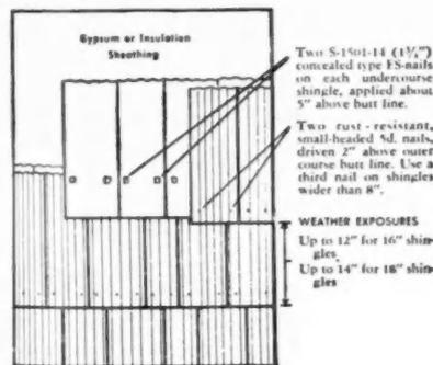
DETAIL showing correct application technique using ES-nails for fastening wood shingles or asbestos shingles to non-wood sheathings. Chart at top is for single course wood shingles; second chart is for double course wood shingles and third for application of asbestos shingles
