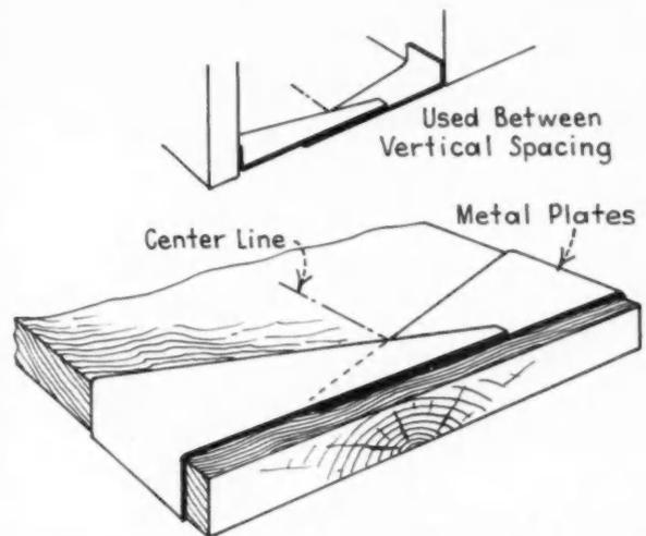
**I**N the position shown in the drawing these plates are used for the purpose of quickly finding the middle distance of any board. By turning them over they can also be useful for indicating the center of two right angle surfaces. They can also quickly find the center between two vertical members.
