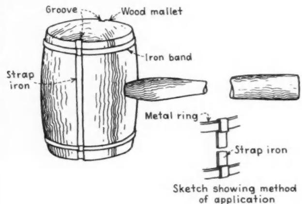
TO prevent metal rings from the head of wooden mallet from working loose and becoming lost, a strap iron was wrapped around ring with excellent results. Groove is cut on both sides of top and bottom of mallet head. An iron band is inserted in each groove. The rings are then placed in position on the head of mallet and the strap irons are bent back over the rings holding them rigidly in position. The strips that bind sheet metal roofing make excellent straps.—Submitted by Oscar West, Bryan, Ohio.
