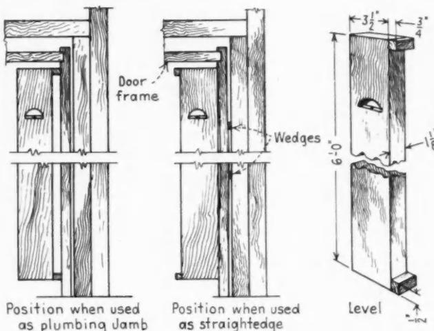
**I**T becomes necessary to carefully plumb the side jambs of door frames to assure accurate fitting and hanging of doors. This can easily be done by applying a homemade straightedge to face of jamb as shown in sketch.
