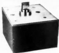
This Pittco Checking Floor Hinge is an engineering triumph. Only 6 3/4" x 6 3/4", it provides positive door speed control, separate checking control, built-in hold-open feature. It's sealed in oil for life. Case and cover are drop-forged. Main working parts are hardened and ground tool steel. Bearings are anti-friction precision-ground.
