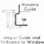
**2 EASY TO ERECT**—The masonry guide and fin make the window easy and inexpensive to install. Guide quickly aligns masonry. Fin ties window rigidly to construction.
