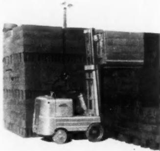
Service-side shifter moves load laterally, enabling operator to spot a cube tight against others without jockeying. Ford-powered. Service Caster & Truck Corp., Albion, Mich.
