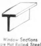
**4 LOW MAINTENANCE**—The window is engineered in hot rolled steel, bonderized and painted. Can't rot or swell. Screen frame is painted, wired with 18 x 14 bronze mesh. Storm panel is insulated with rubber seal and aluminum edging.
