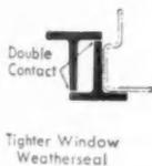
**3 SAVES FUEL**—The window closes tightly because it has double contact weathering. Then, too, the Combination Screen and Storm Panel provides added comfort, saves additional heat.
