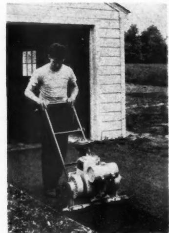
to curbs, rails, manholes, buildings or fences. Requires no water. Impactor plate heated by engine exhaust. Travels under its own power when working. Powered by 2 1/2-H.P. Wisconsin Model AB air cooled engine. Working speed on level ground is 35 to 42 F.P.M., depending on type of material and thickness of mat. Wayer Impactor, Inc., 12, North Third St., Columbus 15, Ohio.
