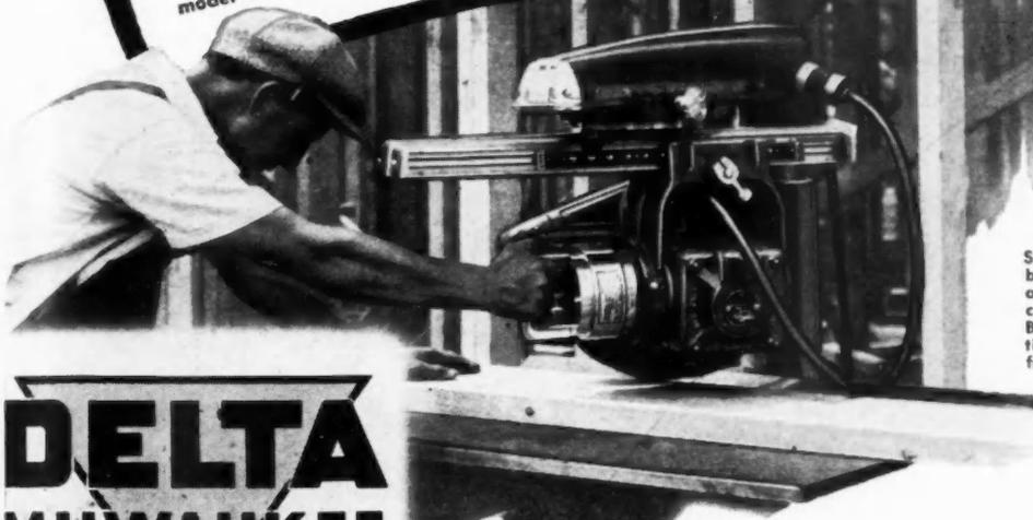
Shown is Delta Multiplex Model 40A with cabinet base. It has a rip capacity up to 3 1/4". Also available is Delta Multiplex Model 30A with cabinet base — and a rip capacity up to 2 1/4". Both models are widely used for cutting foundation forms, sheathing, roofing, cabinets, doors, frames, drawers, sills, stair treads, etc.
