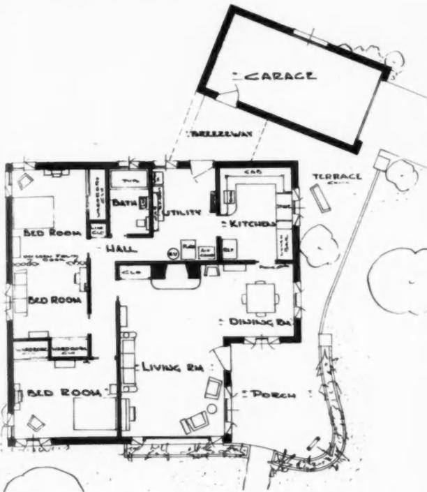
TYPICAL standard plan of Diamond Bar houses. Each is laid out so it is not necessary to cross one room to get to another
