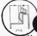
**2** **Weathertight:** Double contact construction (shown at left) blocks wind or rain.
