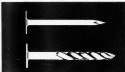
USE these nails for asbestos cement board strip. The center head-nail hole is only for unusual conditions.
