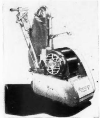
is turned on, it starts under "no-load" condition, due to automatic V-belt take-up. As motor gains speed, pulley squeezes V-belt from side and belt then turns drum. Simple push-button speed control in ranges from 1,600 to 2,800 R.P.M. in 200 R.P.M. gradations. When dial is turned, diameter of drum pulley is changed, varying speed. Easy servicing. Variable drum pressure from 52 to 103 pounds. American Floor Surfacing Machine Co., Toledo, Ohio.
