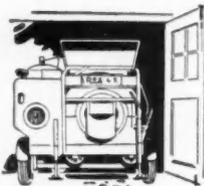
only 87 inches with skip up and 72 1/2 inches with skip down . . . permits working in restricted areas and allows for plenty of headroom for parking in garage or other buildings.
