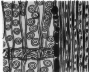
Cedar shingles and shakes have millions of microscopic insulating cells to resist heat transmission.
