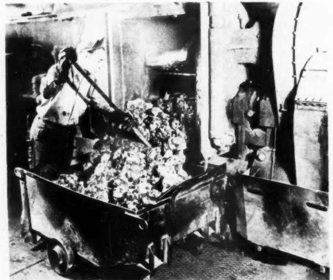
**4.** MOTTLÉ colors for marbleizing are added to the mix a short time before the mixing cycle is completed
