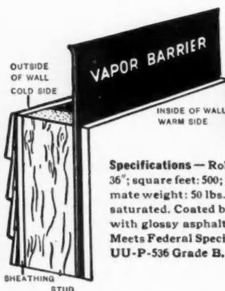
**Specifications** — Roll width: 36"; square feet: 500; approximate weight: 50 lbs. Asphalt saturated. Coated both sides with glossy asphalt surface. Meets Federal Specifications UU-P-536 Grade B.
