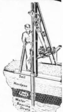
Drill your own wells for that needed water—as many as you need—outside—in the cellar—in the barn. The new improved CONSOL Driller—1948 Model—is equipped with a special replaceable Drill Head. It will drill through many feet of solid rock without re-sharpening. Simple to operate, easy to set up. Do the work yourself at small cost.
