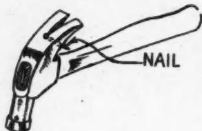
TO SPEED up a job where hundreds of nails are to be removed, and to save removing each nail from the claw of the hammer by hand, allow a nail to get firmly stuck in the "V" of the claw hammer, then there will be no room for another nail to stick.
