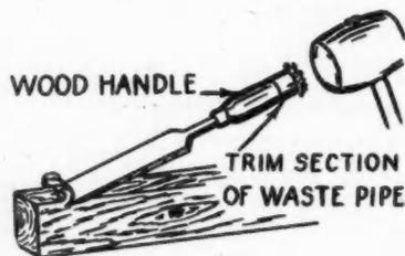
TO KEEP wooden handles from splitting when driven by hammering, use left over ends of plumbers nickel and chrome-plated trim as a band for the end. GEORGE T. MANN, Fort Meyers, Fla.
