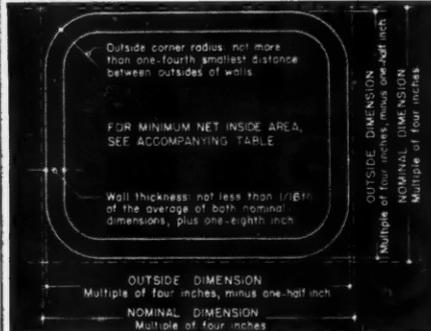
NEW modular dimensions for flue lining in multiples of four inches set up by the National Clay Pipe Manufacturers.
