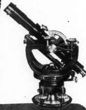
Rugged — accurate — highly dependable, the Universal Level-Transit offers builders an all-purpose instrument of unexcelled practicality and versatility. Quickly converted from a precision level to a highly accurate transit in two easy motions.
