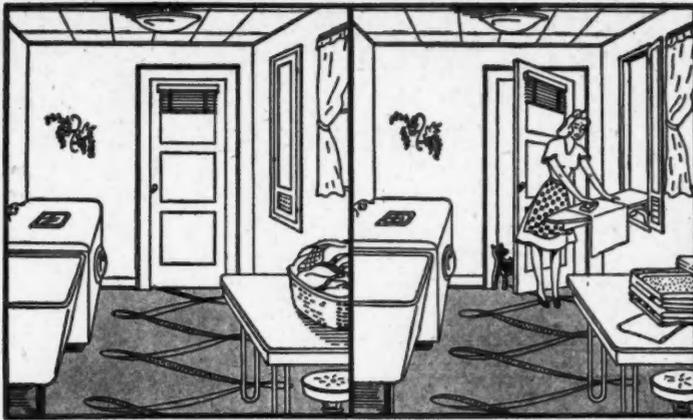
In this utility room there's only one possible place for a modern cabinet-type ironing board — next to the door. The conventional cabinet board would be impractical; could block the entrance, could be used from only one side.
