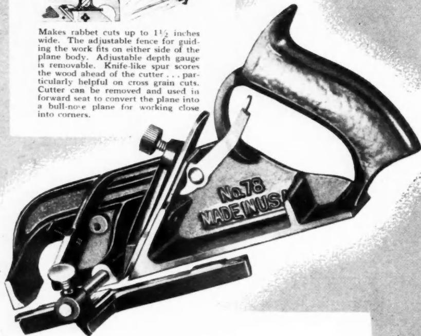
The carpenter's favorite tool for making quick work of rabbet joints for shelving, built-in bookcases, weatherstripping and other fancy rabbeting jobs is the Stanley No. 78 Plane. Makes smooth cuts even across the grain. Simple to adjust and use, the No. 78 Rabbet Plane is just one of the many planes Stanley manufactures to help woodworkers do better work. Stanley Tools, New Britain, Connecticut.
