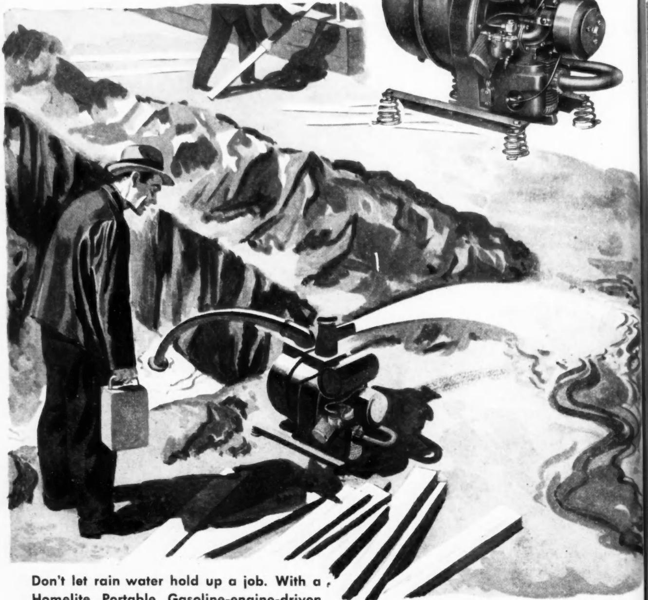
Don't let rain water hold up a job. With a Homelite Portable Gasoline-engine-driven Pump handy you can pump out every drop of accumulated water in a cellar or excavation in practically nothing flat. Self-priming, non-clogging and completely automatic, a Homelite pump has a 28-foot suction lift and will pump up to 15,000 gallons per hour.
