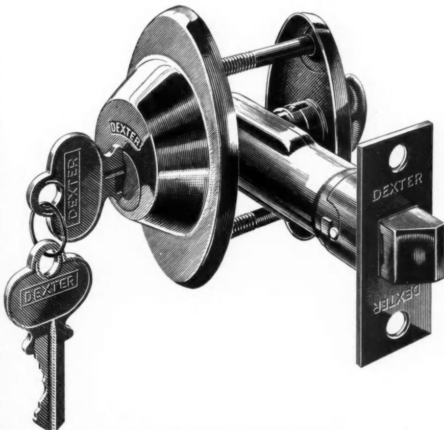
Illustrated: TYPE "E" Five-Pin Tumbler Cylinder Night Latch for grade and rear doors (better appearance than rim lock, installs into—not onto—the door). May be Master Keyed or Keyed Alike with Dexter front door sets.
