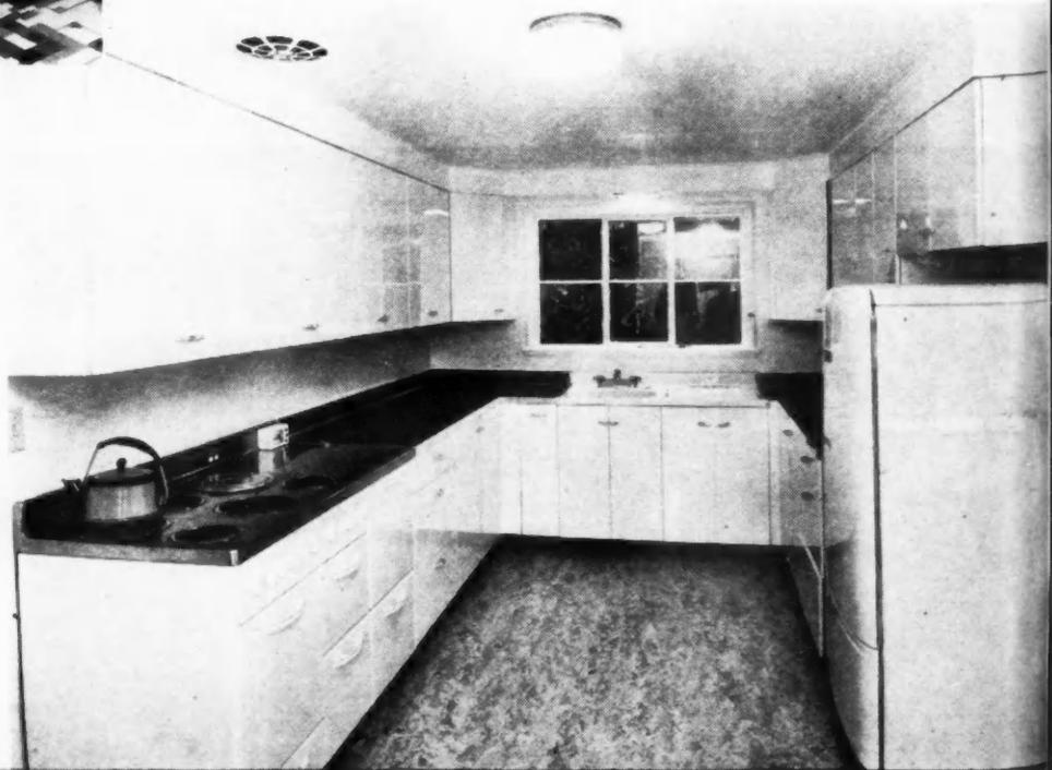
THIS kitchen contains a much-wanted feature—a U-shaped plan, to eliminate extra steps, with continuous working space. There is a ceiling ventilating fan over stove.
