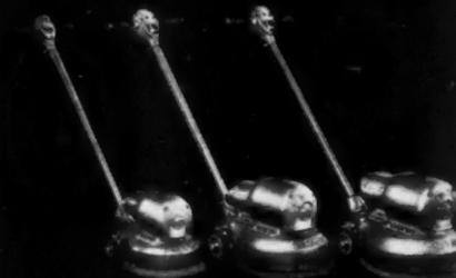
*Disc Sand and Polish*—American Deluxe can be used for disc sanding, steel wooling, polishing and scrubbing. Operates either on wheels or as riding-on-head. Made in three sizes: eleven, thirteen and fifteen-inch discs.
