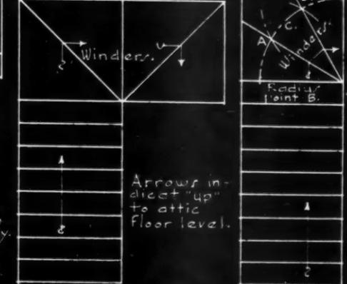
Note: Total run of stairs is distance from face of lower riser to face of top riser measured horizontally; in this detail  $12 \times 8$  or  $8 \times 8$ . Total rise is distance from top of finish floor to top of finish floor; in this detail  $8 \times 4$ . Dividing by number of risers, 13 gives  $7\frac{2}{3}$  or approx.  $7\frac{1}{2}$  for each riser.
