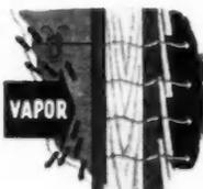
Continuous insulation is provided at the floor line and foundation framing, at the top plate and rafters, and at corners. Insulation at these points is highly important to block drafts and stop "heat leaks."
