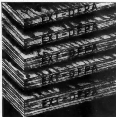
Exterior type plywood, easily identified by the "grade trademark" shown above, is made with completely water-proof synthetic resin binder. For outside siding 3/8" thick, Sound 1-Side grade of Exterior plywood is generally specified. Exterior type plywood (EXT-D.F.P.A.) should be specified for all permanent outdoor use and for interior use where moisture conditions are present.
