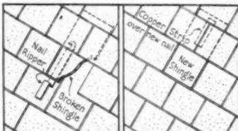
METHOD OF REMOVING AND REPLACING BROKEN AMERICAN METHOD SHINGLES
