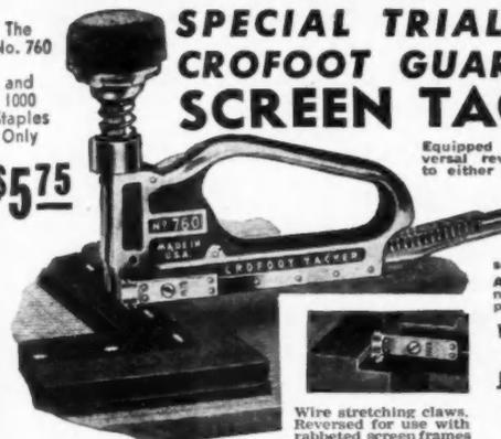
Equipped with a set of universal reversible claws, used to either pull or push screen wire tight. A down stroke on the plunger drives a two-prong steel staple into the frame, holding screen wire firmly.
