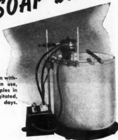
To make sure Monowall can withstand severe conditions in use, Armstrong submerges samples in a tank of constantly agitated, hot soap solution for 8 days.
