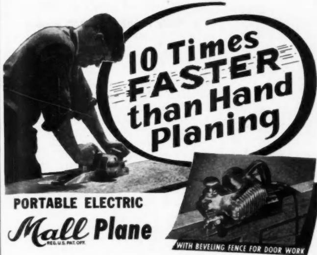
The operator simply guides the plane across the work and the heavy duty motor does the rest. MALL Planes make cuts up to  $\frac{1}{4}$ " deep and  $2\frac{1}{2}$ " wide in both pine and hardwood with speed and precision. The cutter is under constant control and can be raised or lowered while cutting to vary depth of cut. A hairbreadth adjustment 0" to  $\frac{1}{8}$ " is easily made by turning the handle.
