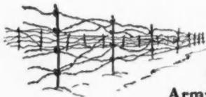
A unique CECO production line twists Ceco reinforcing bars into Army screwposts. Screwposts that, when strung with barbed wire, stand grim sentry duty in jungle outpost and German field.
