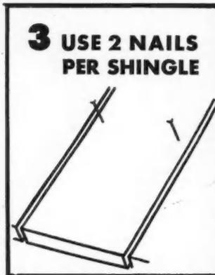
**WHY?** Two nails are sufficient. Additional nails restrict expansion and contraction of shingles. Nails should be driven approximately 3/4 of an inch from each edge of shingle and about 1 1/2 inches above butt line of shingles to be applied in next layer.
