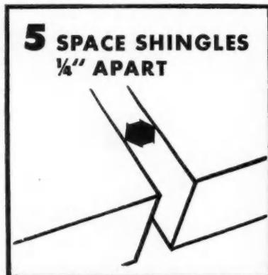
**WHY?** This spacing allows adequate room for the shingles to expand during rainy weather. It also permits ready drainage and dissipation of moisture. These joints must not line up in successive courses of shingles.
