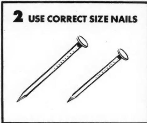
**WHY?** Nails must conform to the thickness of the shingles on the roof. For 16-inch and 18-inch shingles, use 1 1/4-inch (three-penny) nails. For 24-inch shingles, use 1 1/2-inch (four-penny) nails. Be sure that nails are rust-resistant. When shingles are nailed as directed in No. 3, the overlapping of the succeeding courses completely covers the nails and protects them from the elements.
