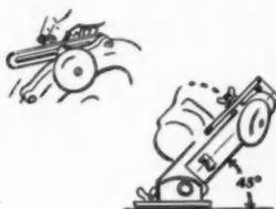
Simple depth adjustment. Notched base makes it easy to follow cutting line.
