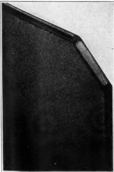
CORNER shown cut off to make clear inner structure of new Celotex siding.
