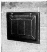
Majestic Grade Line Chutes (at left) put the exterior opening on the grade line. Built for hard service. Special door flange makes this chute practically watertight. Gravity latches operate with chain and pull cord. Body angle iron re-enforced at edges and corners. Finished in rust resisting asphaltum.
