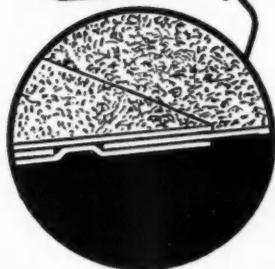
Adequate projection of shield beyond wall or pier is most important.
