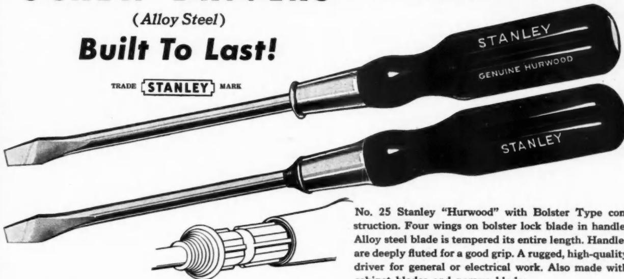
No. 20 Stanley "Hurwood" Screw Driver. Forged alloy steel blade goes all the way through handle and is locked in place by two projecting wings and a rivet through ferrule, handle and blade. A popular driver for all-around work. Also made with cabinet blades.
