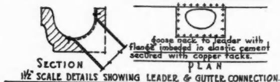
SECTION 1/2" SCALE DETAILS SHOWING LEADER & GUTTER CONNECTION.
