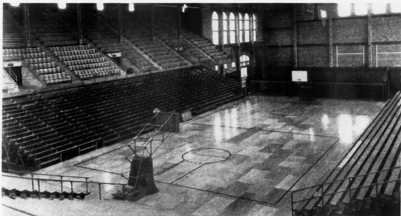
THE University of Washington basketball floor of Douglas fir plywood laid on the ground in the Campus field house at Seattle, Wash. In spite of this severe service, these panels have been relaid season after season without apparent depreciation.
