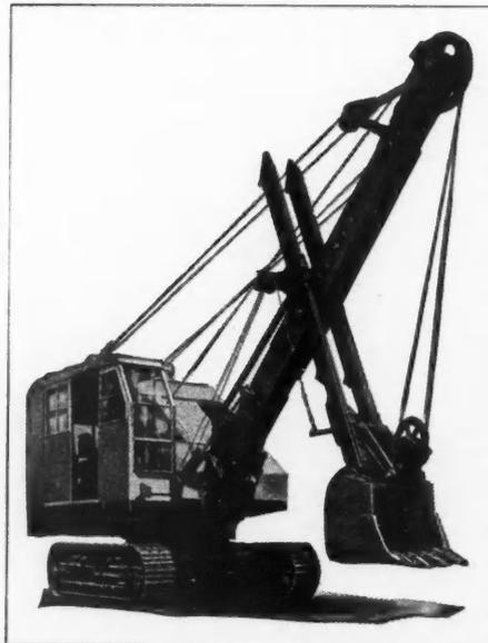
ALL-PURPOSE excavator of high tensile steel for weight reduction and greater strength.
