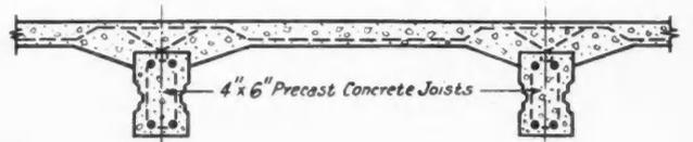
TYPICAL SECTION THROUGH JOISTS AND SLAB
