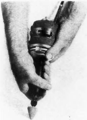
High speed grinder gets into irregularly shaped holes and hard to reach places.
