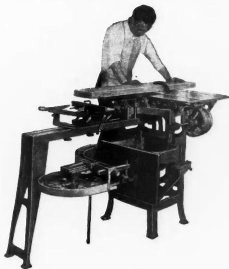
Cross cutting with the Electric Carpenter—band saw lowered to horizontal position.
