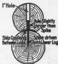
At left — log spiking detail used by Wilcox. At right — rig used to handle logs on job.
