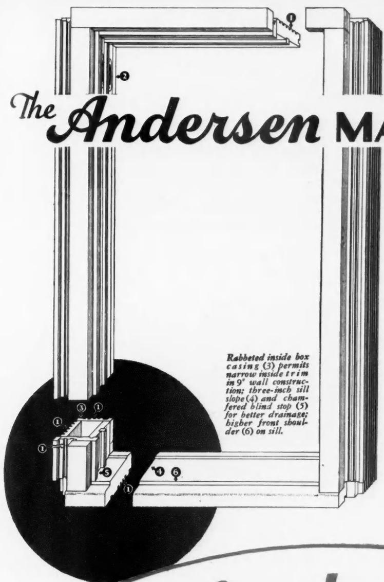
Mortar clinch grooves (1) on all surfaces making contact with masonry make the frame practically self-caulking; Andersen patented noiseless sash pulleys (2) now have machine-turned wheels.
