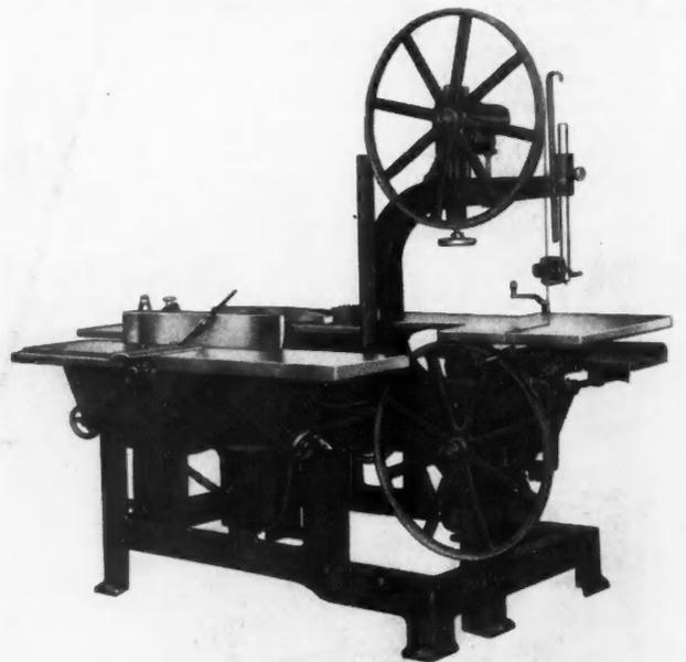
A Universal Woodworking Machine Which Eliminates the Use of Clutches for Starting and Stopping.
