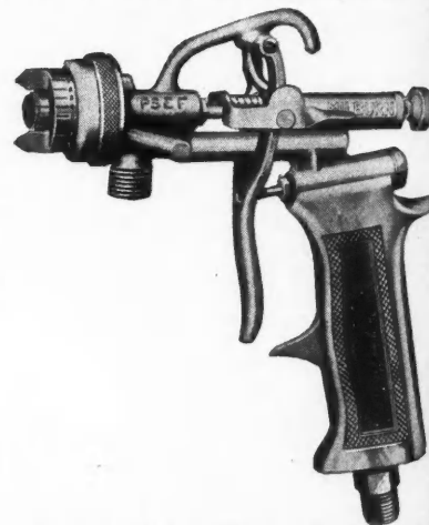
Two Additions Have Been Made to This Paint Spray Gun Which Give the Operator Complete Control of the Spray.
