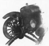
A Light, Powerful Pump Which Can Be Quickly Connected or Disconnected When Mounted on the Truck,
