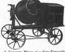
A Concrete Mixer of a Size Especially Adapted to General Construction, Foundation and Sidewalk Work in an Improved Model.
