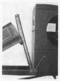
This Simple, Reliable, Hand Hoist Increases the Range of Use of the Ford Steel Truck Body.
