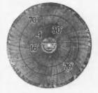
Outer line on this recording thermometer chart shows constant temperature downstairs, day and night, for the entire week ending Feb. 7. Inner line shows outside temperature varying from 16° to 4° to 30° above zero.
