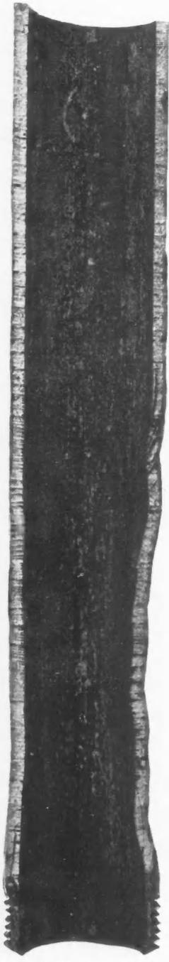
Piece of pipe referred to in the accompanying letter. Note full threads and full thickness of the wall throughout the length. Also the softness of the pipe as evidenced by the crushing of the sides with the pipe tongs when removing it. The roughness on the inner surface is a slight scale formation and not corrosion.
