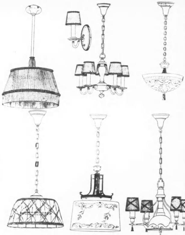
Some Well Designed Dining Room Units. It Is of Interest to Note the Tassel at the Bottom of the Semi-Indirect Bowl. This Conceals Half of an Attachment Plug for Use with Cooking Devices. The Wicker Dome Carries an Opalescent Reflector Indicated by Dotted Lines.
