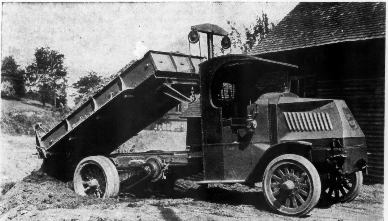
Dumping the 3½-Ton Dump Truck Which Saved \$60 a Day for the Dempster Construction Company, Knoxville, Tenn. This Truck Made Thirty-four Trips Daily and Earned \$130. Their Work Required Backing Down a 15 Per Cent Grade to the Bottom of a Hollow 30 Feet Deep.
