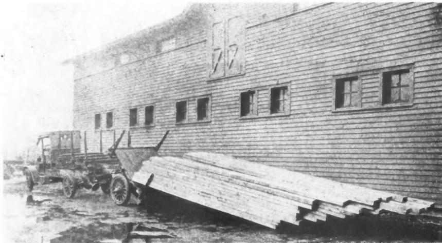
Second Stage in Operation. The "Trailmobile" Has Opened Up Like a Jack Knife While the Load Is Nearing the Ground.
