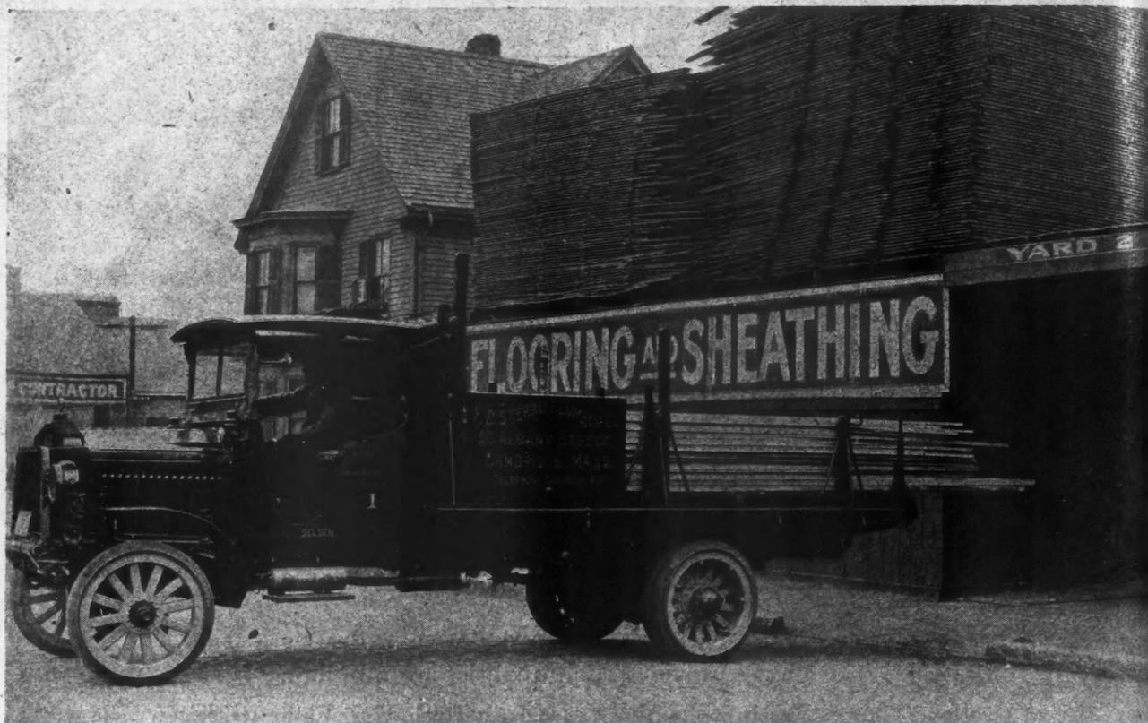
F. D. Sherrit Lumber Co., Cambridge, Mass., Make a Specialty of Flooring and Sheathing and Naturally During This Busy Building Season Are Going at Top Speed. This 3½-Ton "Selden" Truck, Equipped with a Special Roll Body for Unloading Lumber, Has Been Doing Great Work for Them All Season.
