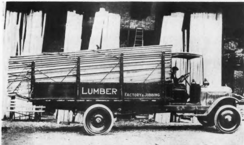
The "Republic" Truck of James E. Tague & Co., Lumber Dealers, Loaded, Ready to Start for the Building Job. This Truck Carries More Than Three Times the Capacity of a Wagon and Has a Speed of 15 Miles an Hour When Loaded. It Is Easy to See Why Motor Trucks Are an Essential Part of the Equipment of Successful Lumber Dealers.
