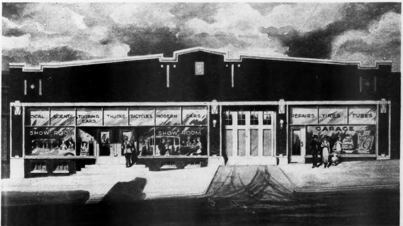
Front Elevation of Building Designed to House the Modern Automobile Sales Agency. Show Room for the Machines, a Salesroom for Accessories, Office and a Large Garage Are Provided in This Building. It Is 75 by 100 Feet in Dimensions, of Brick Construction with a Trussed Roof, and Has an Attractive Front of Face Brick and Terra Cotta.
