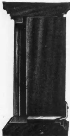
Fig. 1. A Simple Pattern of Single Rib Strip that Fits Into a Groove Made in the Sash.
