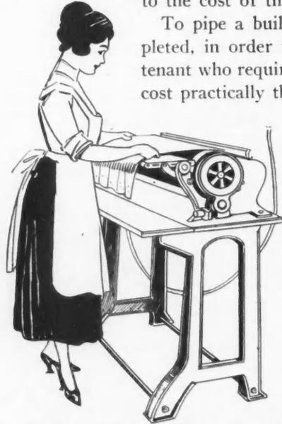
A Mangle, Heated with Gas, Does Away with Much of the Labor of Ironing the Flat Clothes.
