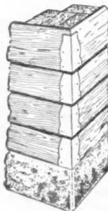
will enable even inexperienced workmen to make perfect "mitred" corners quickly. Pierced ready for nailing, they save beveling expense, fit any corner and are practically invisible when painted. Made of heavy galvanized iron, they form a neat, indestructible and weatherproof corner.
