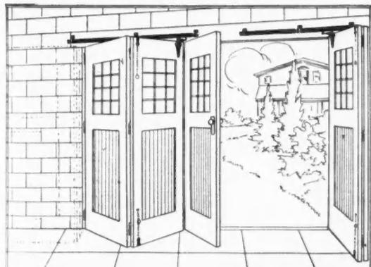
Illustration at left shows No. 58 Clozite Hanger on private garage doors opening inward. Center door used as separate entrance. Illustration below shows No. 78 Clozite Hanger on big heavy factory doors, opening outward. Center door used as separate entrance.
