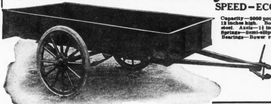
Capacity—2000 pounds. Body—8 feet long, 46 inches wide, 12 inches high. Body and under frame built of open hearth steel. Axle—1½ inch square rod, special high carbon steel. Springs—Semi-elliptic, oil tempered and double heat treated. Bearings—Bower roller. Wheels—1½ inch spoke, artillery type, second growth hickory. Tires—32x2, solid rubber. Weight—534 lbs.
