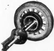
The Torbensen Internal Gear Drive, used in all Republic Trucks, delivers 92% of the motor power to the wheels. We know of no other type of drive that delivers as much. The entire load is carried on a separate I-beam axle. The driving mechanism has nothing to do but drive the truck.
