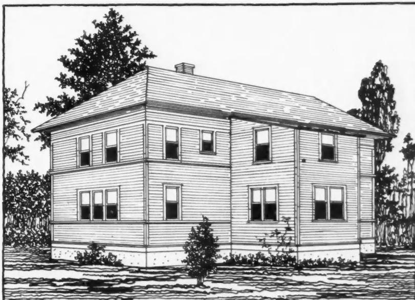
An Improper Way to Roof an Extension to a Hipped Roof House.
