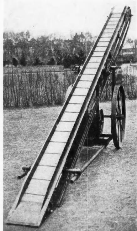
Close Up View of Portable Scoop Conveyor.
