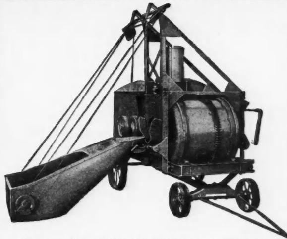
Lansing No. 7 "One-Bag" Mixer with Power Loader and Water Tank
