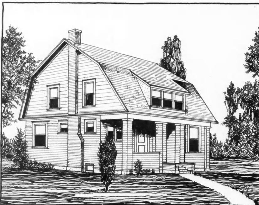
Flat Dormer on Gambrel Roof Continues Upper Roof Slope Without a Break.
