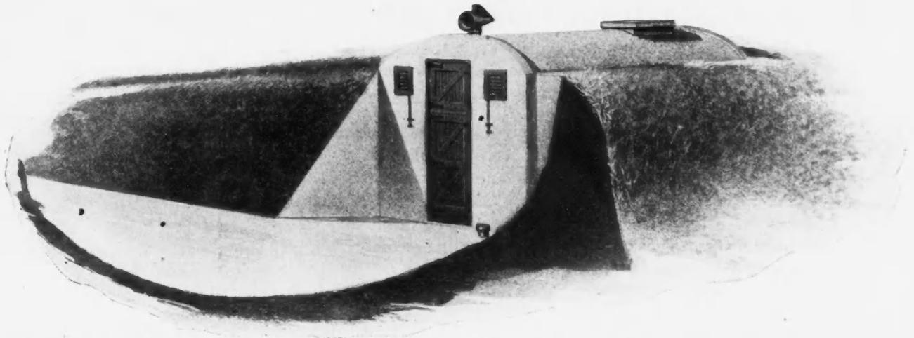
Perspective Sketch of Vegetable Storage Cellar of Concrete Construction. The Near Embankment is Shown Cut Away So That the Driveway and Door May Be Seen. Complete Working Plans for This Valuable Food Storage Building are Presented in the Blue-Print Page Opposite.
