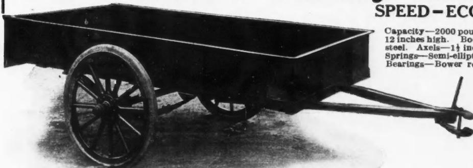
Capacity—2000 pounds. Body—8 feet long, 46 inches wide, 12 inches high. Body and under frame built of open hearth steel. Axles—1½ inch square bed, special high carbon steel. Springs—Semi-elliptic, oil tempered and double heat treated. Bearings—Bower roller. Wheels—1½ inch spoke, artillery type, second growth hickory. Tires—32x2, solid rubber. Weight—534 lbs.
