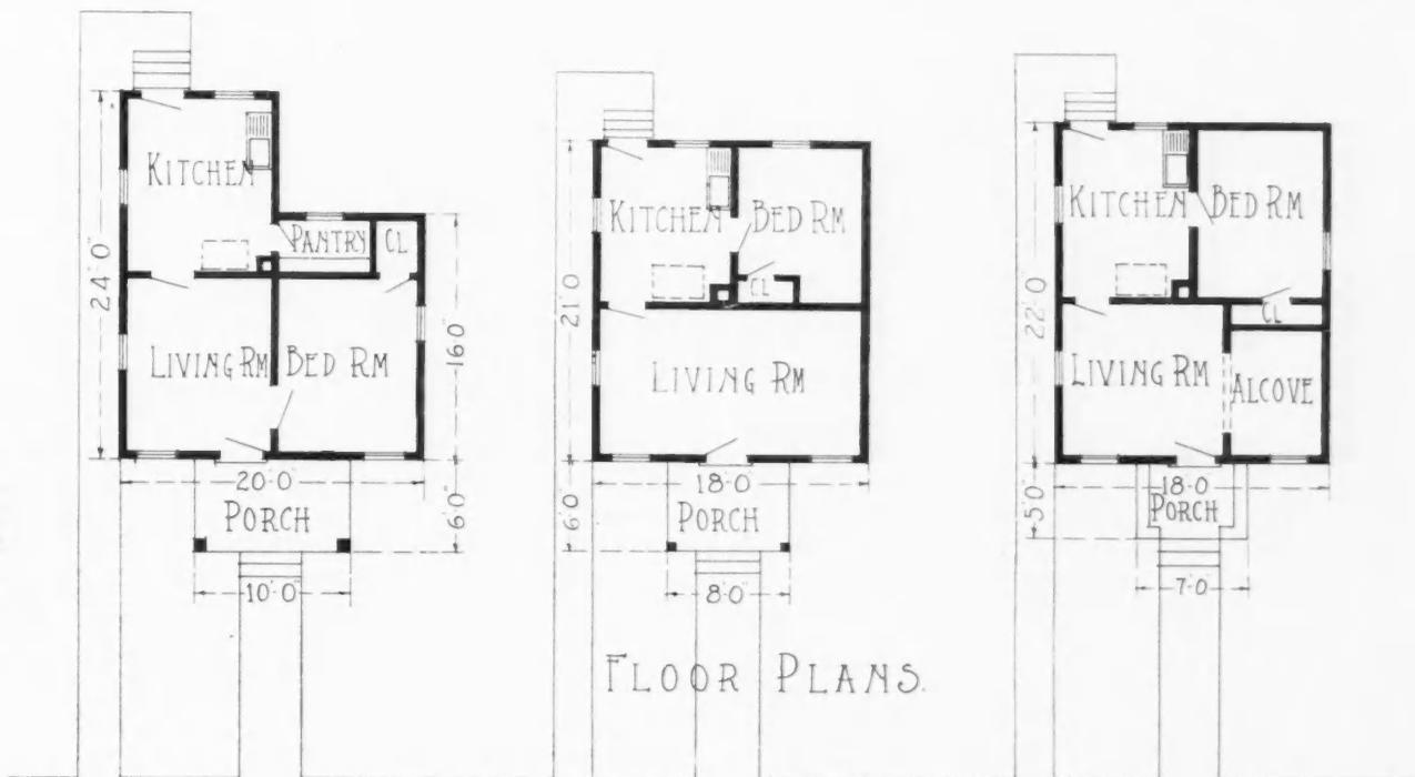
These Three Houses are Smaller, Containing Three Rooms Each. They are 20 and 18 Feet in Width.
