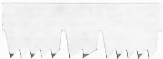
Tooth Detail of New Double Duty Saw.
